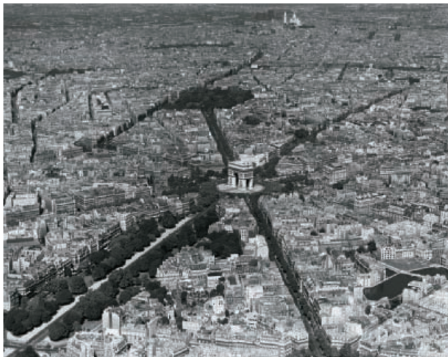
PARIS REBUILT. Baron Haussmann, prefect of Paris under Napoleon III, presided over the wholesale rebuilding of the city, with effects we still see today. The Arc de Triomphe, seen here in a photograph from the 1960s, became the center of an étoile (star) pattern, with the wide boulevards named after Napoleon I's famous generals.
