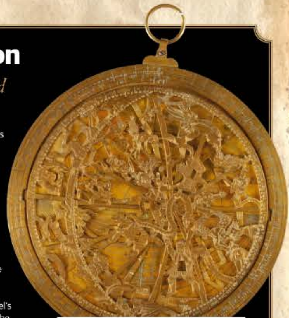
A 16th-century brass astrolabe, which was used to establish latitude by measuring the angle of the Sun to the horizon
