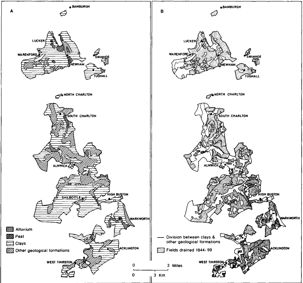
Figure 3.15 Land drained, 1844–1899, and drift geology, the duke of Northumberland’s Alnwick, Lucker, Shilbottle and Warkworth bailiwicks (Sources: Northumberland MSS: Draining vols., 1–3; T. Bell and sons, Survey... of the Northumberland estate, 1850, map nos. 1–102; Geological Survey, 1 in drift sheets 4, 6 and 9)
