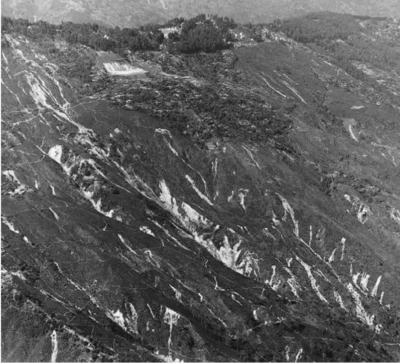
Figure 6.7 The Darjeeling rainstorm of October 1968 was a 50 to 100-year event and produced thousands of landslides. Many were small, yet entire mountain sides were mutilated and only foot travel was possible for many weeks. Within a few years, however, most of the landslide scars had been obscured by natural revegetation, November 1968.
