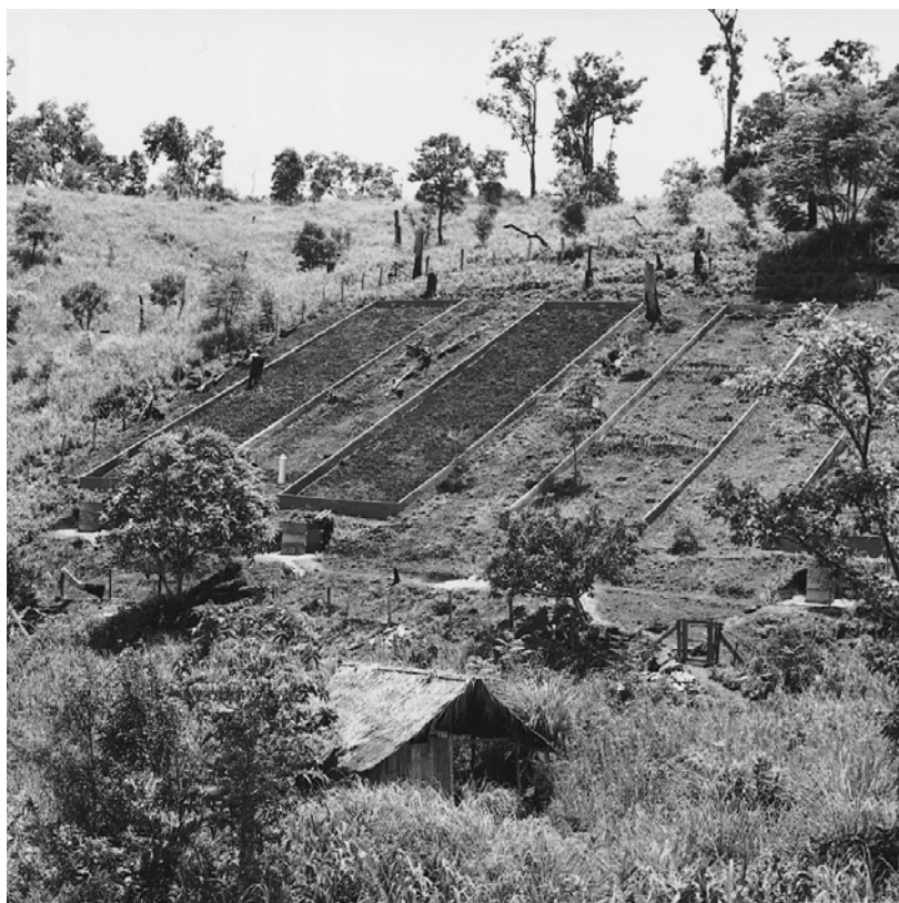
Figure 4.2 The main soil erosion test plots constructed by the UNU–Chiang Mai University research project under the supervision of Hans Hurni, University of Berne, Switzerland (see text for explanation), July 1981.
