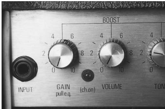
Figure 15-5: The preamp section of an amp.
