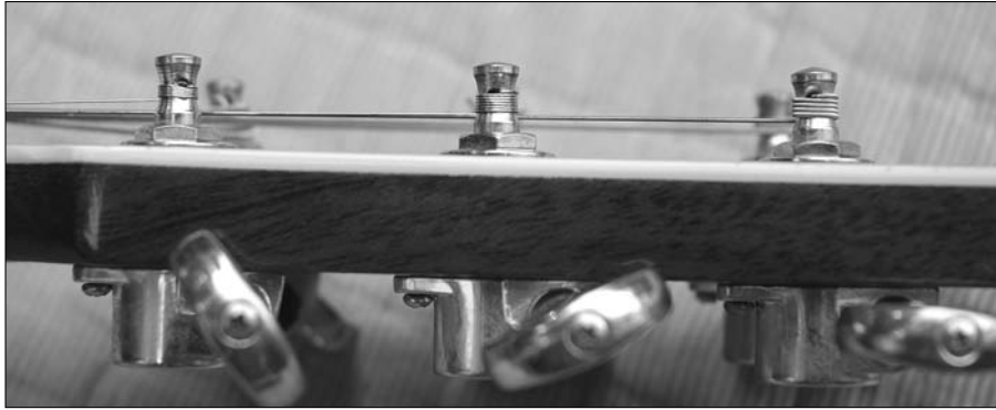
Figure 16-4: Coiling the string on the post.
