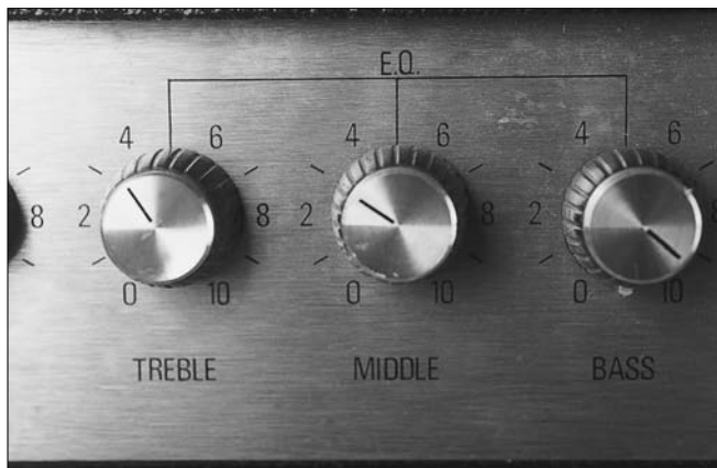
Figure 15-6: The tone section of an amp.
