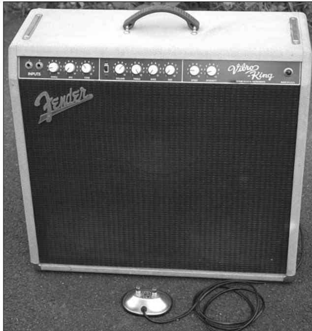
Figure 15-8: An amp with a footswitch- activated boost.
