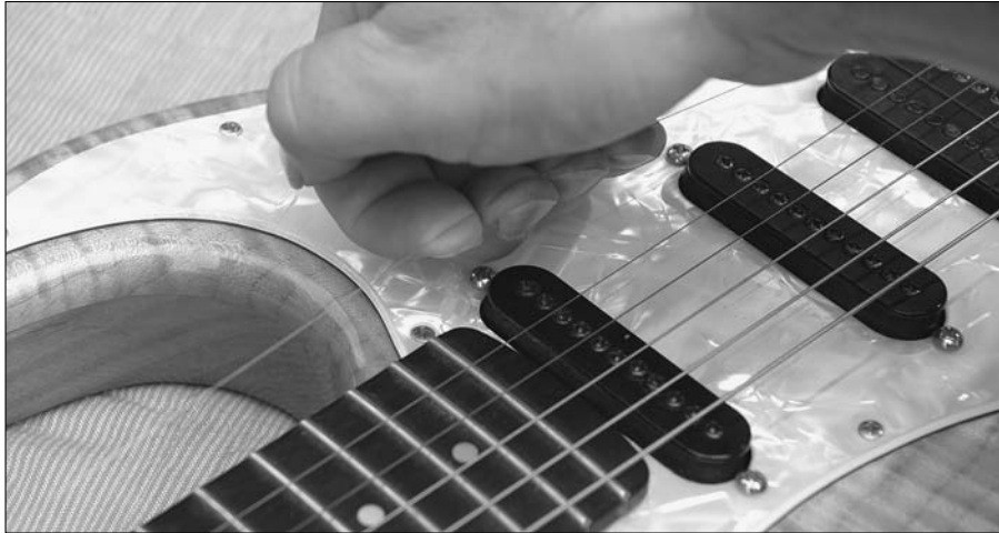
Figure 16-10: Pulling on the string after it's tuned up to get the “stretch” out.
