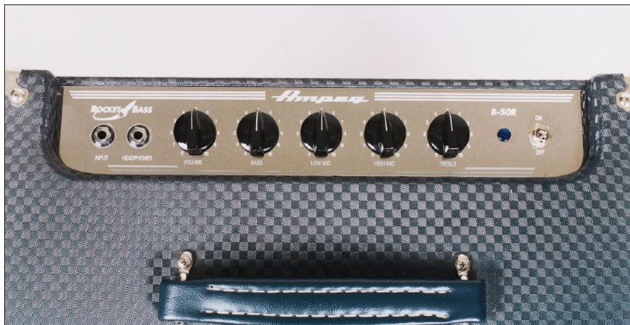
Figure 15-2: The control panel of a bass amplifier.
