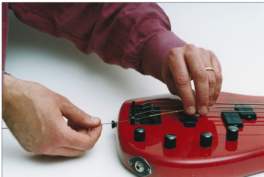
Figure 16-4: Pulling the string through the bridge.
