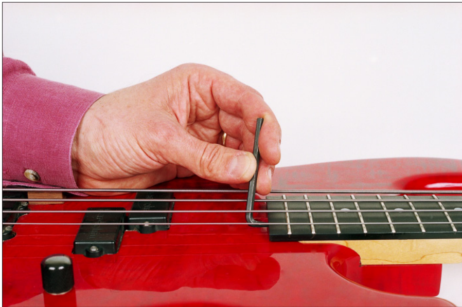
Figure 17-2: Adjusting the truss rod.
