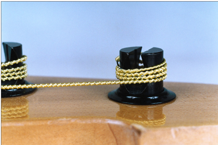
Figure 16-7: Windings of a string at the tuning post.
