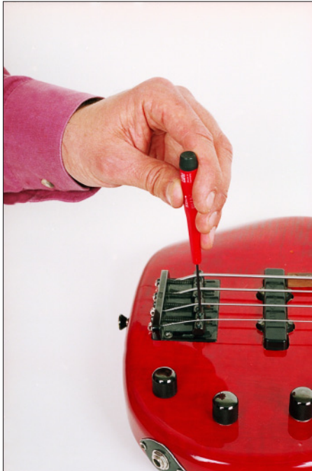
Figure 17-3: Adjusting the height of the saddles.
