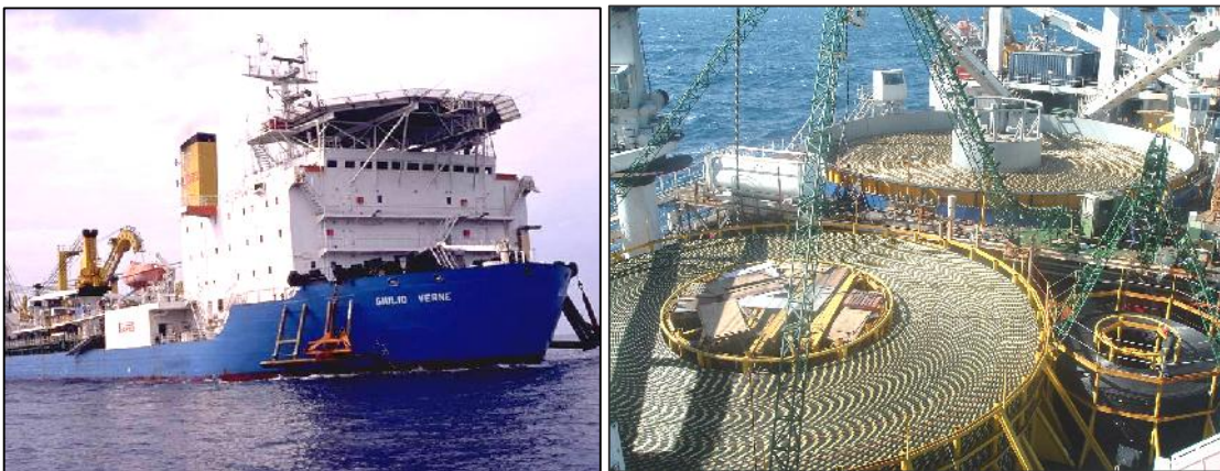
Figure II.1: Cable-ship transporting long lengths of submarine HV cables accommodated in platforms
