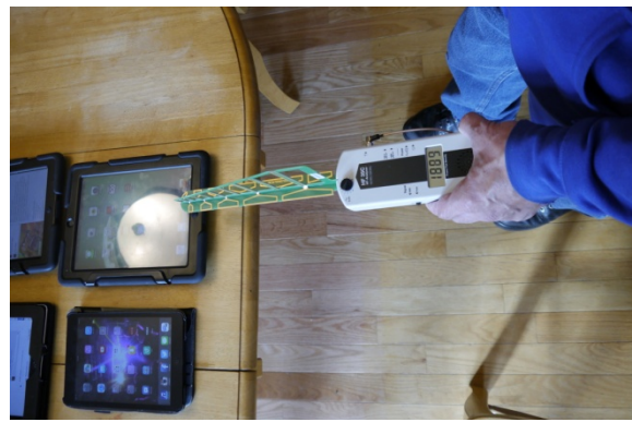
2 ACS iPads, 3 privately owned iPads, 1 cell phone, and 1 smart phone simply turned on. Notice the cumulative effect without purposely accessing the WiFi. Reading 1889 microWatts/cm 2 .
