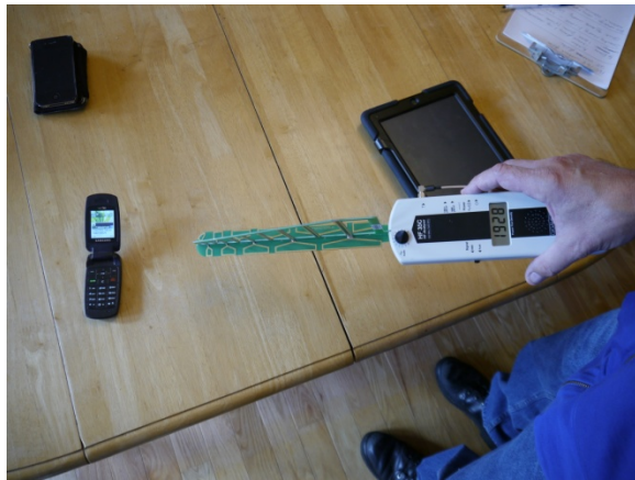
Reading from flip-top cell phone when sending or receiving, 1928 microWatts/cm 2 pictured at 8". Measurements from the flip-top were generally over 2,000.
