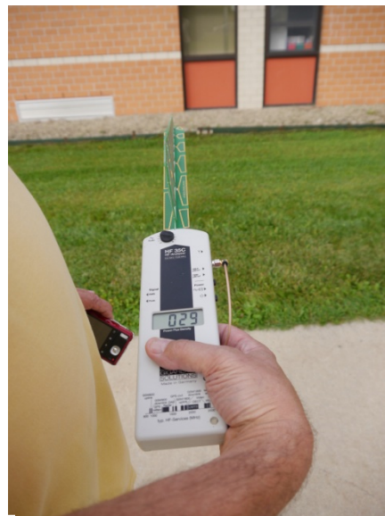
Reading of 029 microWatts/cm 2 near the main office of Orchard Primary School
