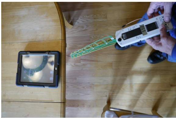
Measuring 598 microWatts/cm 2 from an ACS issued iPad simply turned on.
