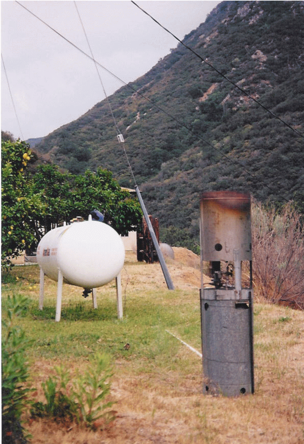
Figure 4. Manually Operated Cloud Seeding Generator and Propane Tank
