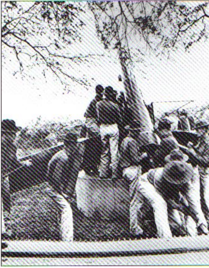
The mobile 155mm guns received after World War I made an important contribution to upgrading the beach and landing defense capabilities. This gun is being manned by the 55th Coast Artillery, and is emplaced on a Panama Mount – a simple concrete pad within a circular ring allowing quick traverse on a stable firing platform. (AM)
