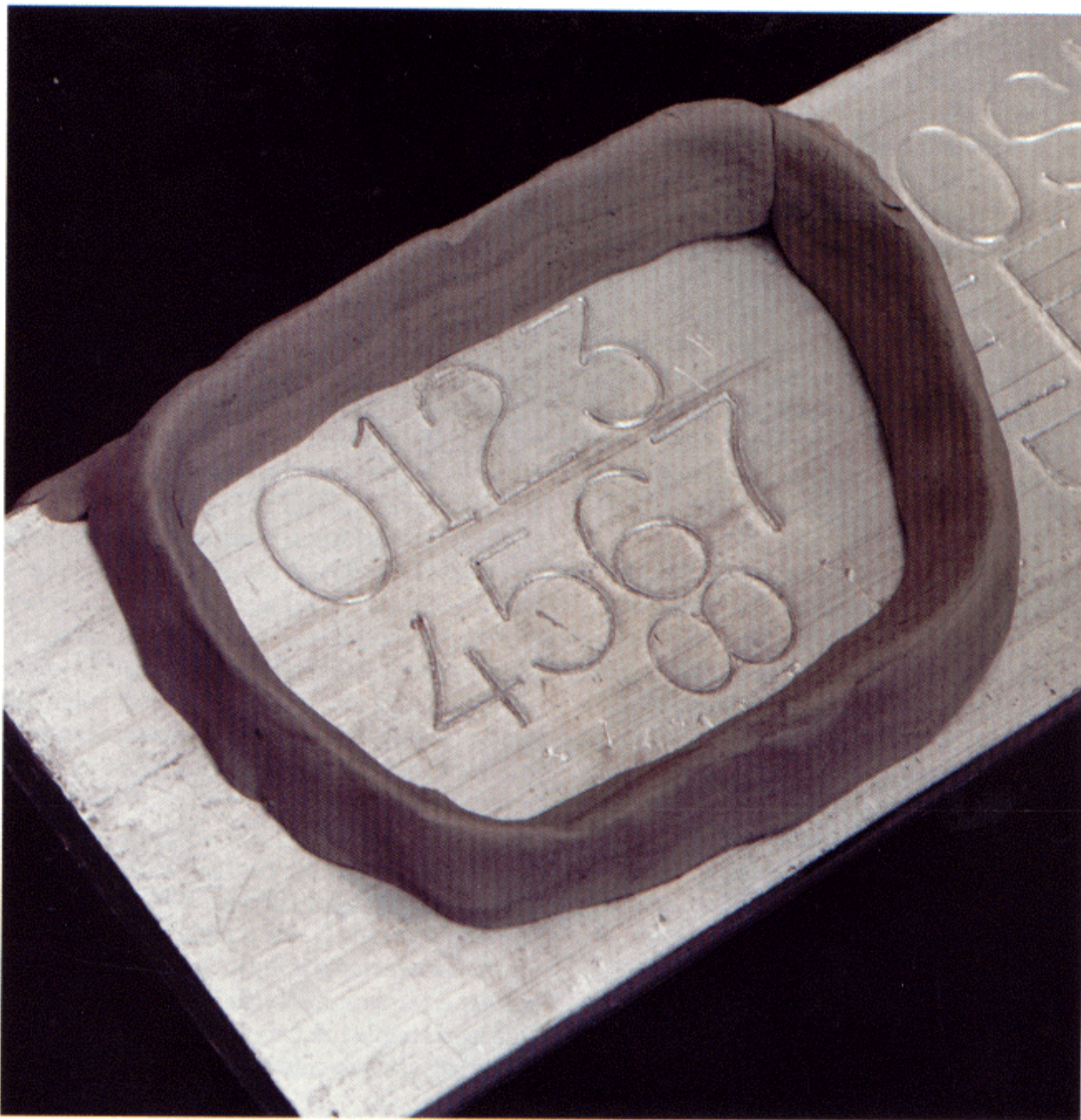
Stamped numbers in metal ready for a plastic cast/impression
