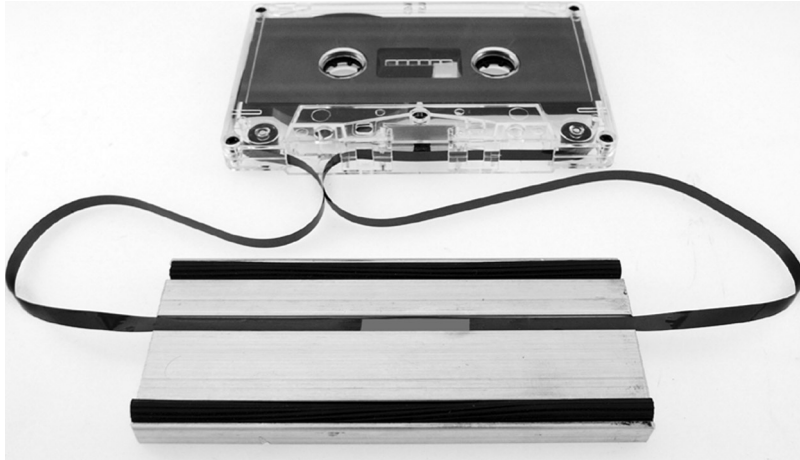
Figure 20.4 Cassette tape splicing
