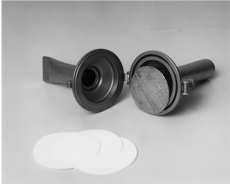
Figure 1.5 The forensic science laboratory stainless steel vacuum nozzle opened view depicting debris trap – Photographer: Horswell
