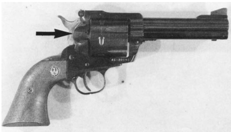
Figure 1.3 Solid-frame revolver with loading gate swung open. Arrow points to loading port where individual cartridges are inserted.
