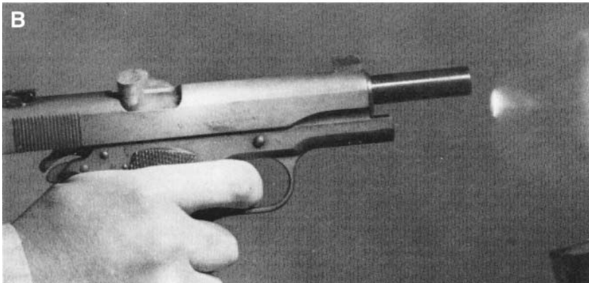
Figure 1.4 (A) The weapon has just been fired. The slide has begun to recoil with the bullet a few inches in front of the muzzle. (B) The slide has recoiled all the way back. The fired cartridge case is being ejected and the gun cocked. The slide will now come forward, chambering a new round.
