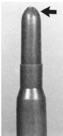
Figure 10.18 Plastic blank with breaking points on top.
