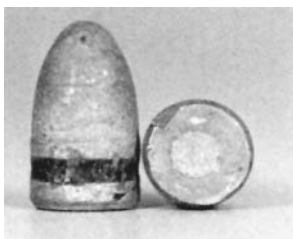
Figure 10.7 9-mm cast bullet showing circular mark on base resulting from sprue.
