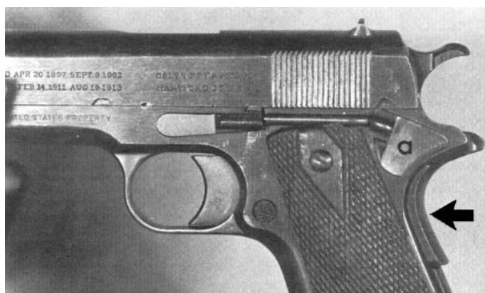
Figure 1.7 Left side of Colt .45 automatic pistol with manual safety and grip safety (arrow).
