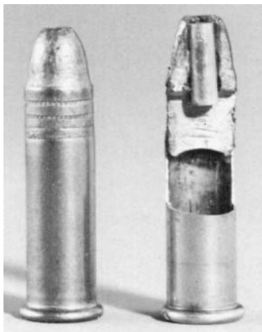
Figure 10.14 Longitudinal section through .22-caliber exploding round.
