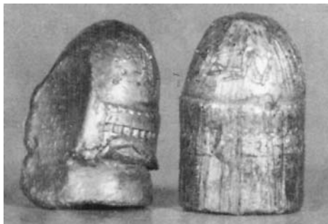
Figure 10.5 The bullet on the left is shortened, shows the absence of rifling, and has one side sheared off compared to the bullet on the right which emerged from the barrel.
