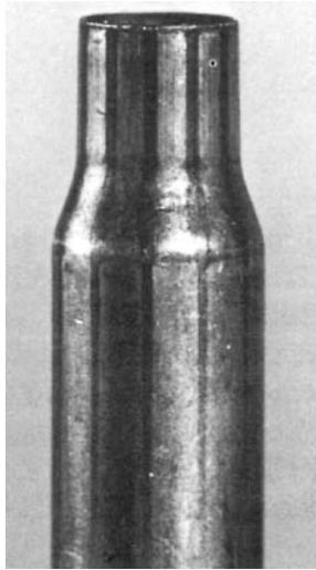
Figure 2.6 Markings on rifle cartridge case due to fluted chamber.
