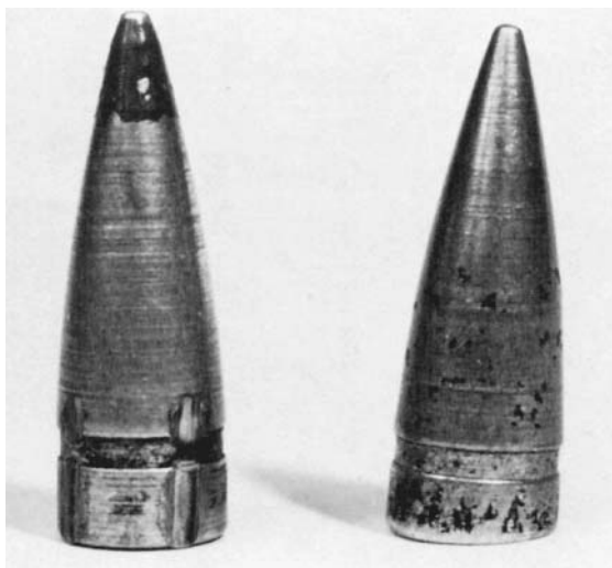
Figure 10.16 Military duplex round. Note the canted base of bullet on right.
