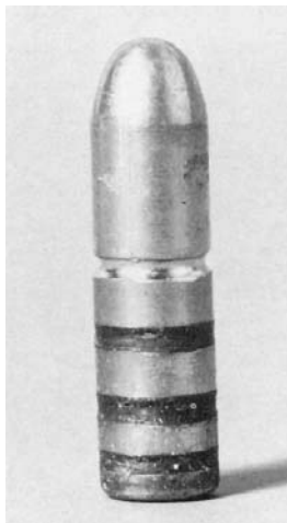
Figure 7.1 Cast rifle bullet with deep cannelures filled with grease.
