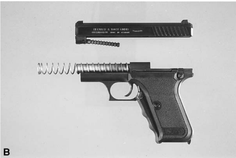
Figure 1.5 (A) Heckler-Koch P7 9-mm pistol with squeeze cocker constituting front portion of grip; (B) Disassembled with piston visible and projecting downward from end of slide.
