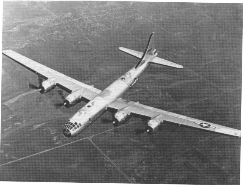
A Boeing B-29, equipped with 4 Wright engines.
