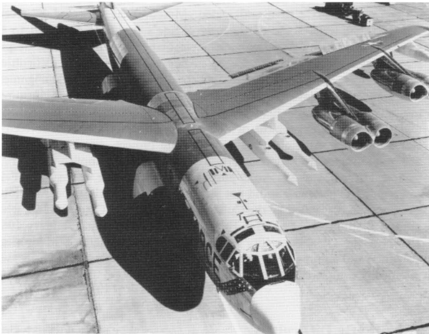
A Boeing B-52H, equipped with 4 Douglas GAM Skybolt ballistic missiles.
