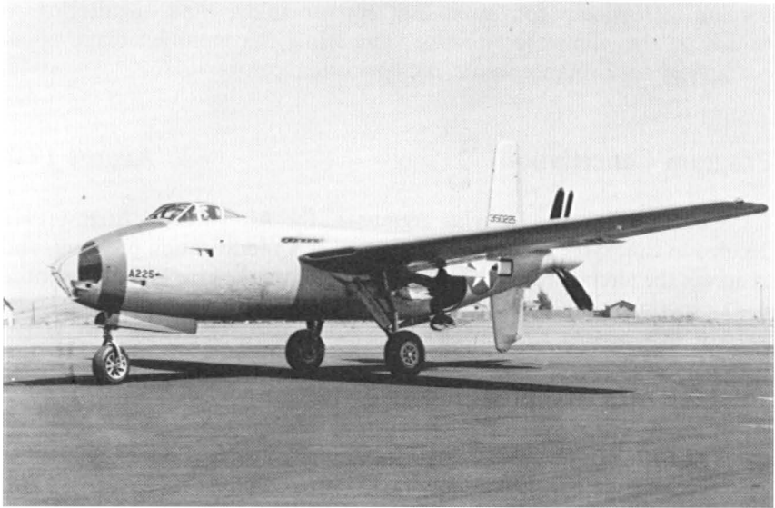
The XB-42 featured a novel engine-propeller arrangement.
