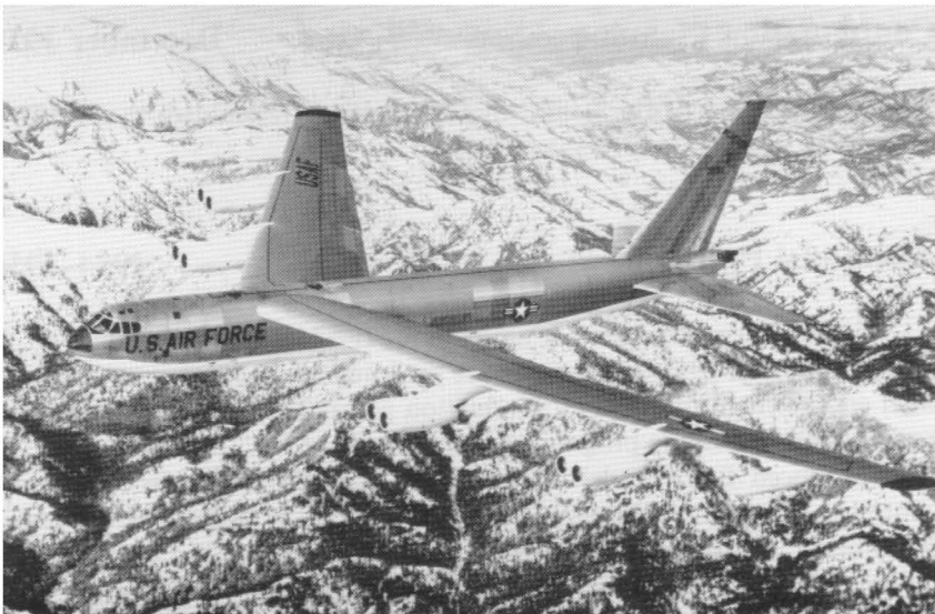
A Boeing B-52C in flight, its under surfaces coated with white thermal reflective paint.
