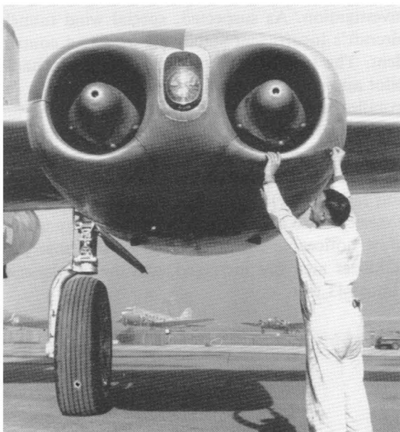
Close-up of 2 of the 4 jet engines that powered the XB-45.
