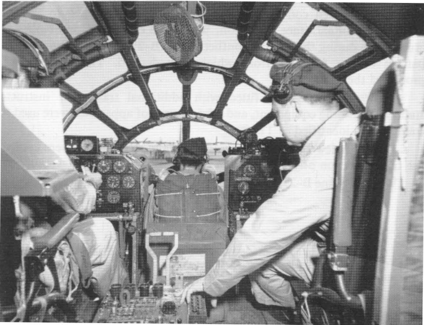
The forward compartment of the B-29 housed the bombardier (front), pilot (left), and co-pilot (right).
