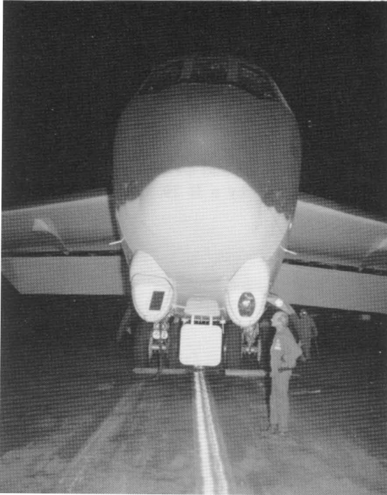
Front view of a B-52, showing the television sensors of the new electro-optical viewing system developed to enhance low-level flight.
