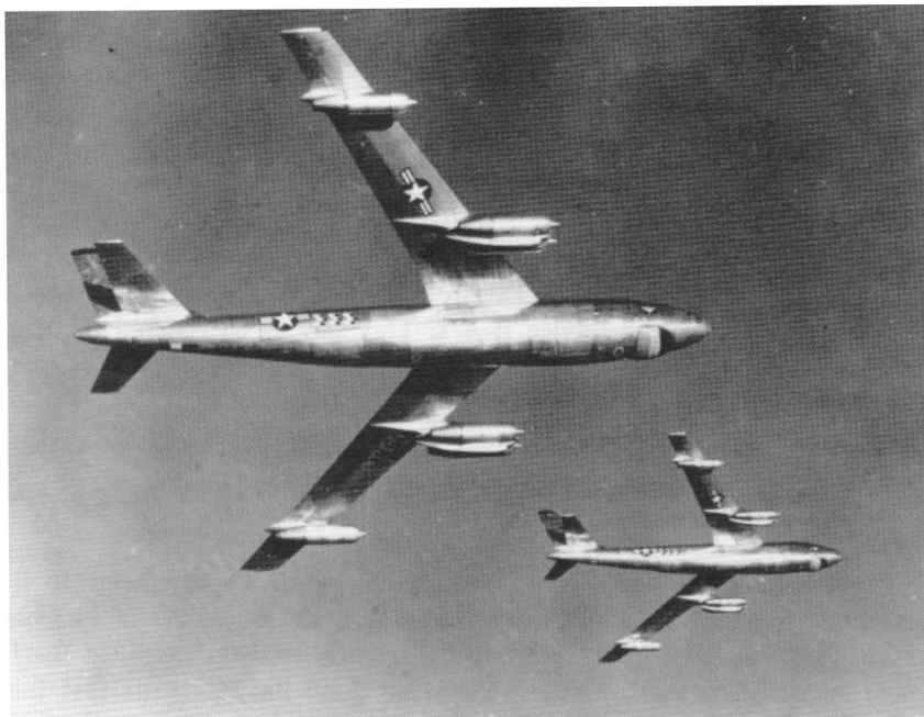
Two B-47Bs, equipped with 6 J47-GE-23 engines.
