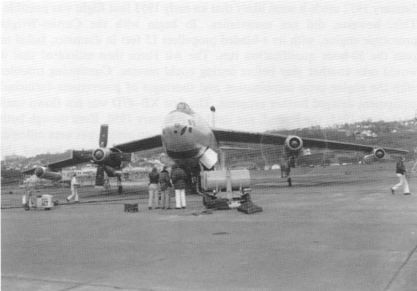
A specially modified Stratofortress—the XB-47D—was used to test the Curtiss-Wright YT49 turboprop engine.
