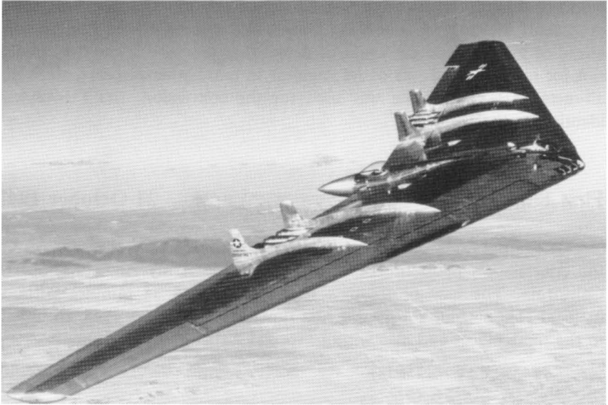
The Northrop YB-49 was a converted YB-35, with jet engines instead of propellers.
