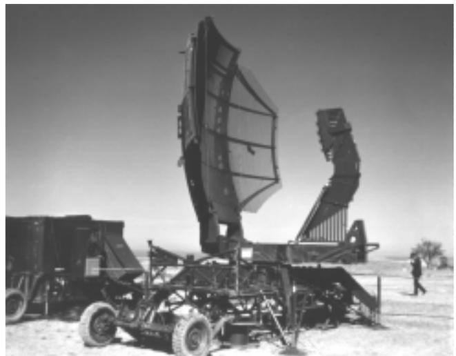
**Figure A76** AN/TPS-43 stacked-beam reflector antenna.
