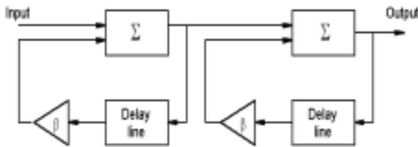
Figure 14 Two-cycle integrator.
