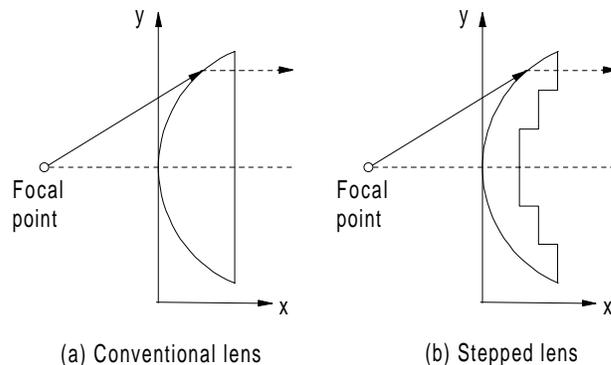
Figure A65 Lens-horn geometry (after Currie, 1987, p. 541).
