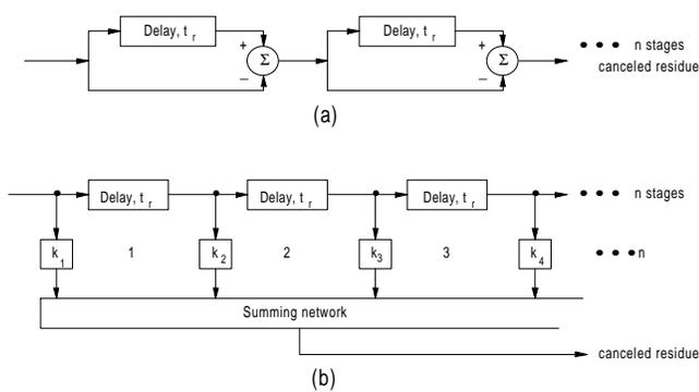
**Figure C6** Multiple-delay cancelers. (a) Cascaded canceler sections; (b) weighted summer (after Nathanson, 1969, Fig. 9.7, p. 328).
