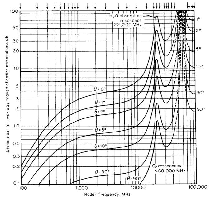
**Figure L17** Total earth-based radar attenuation (two-way) vs. frequency for target outside the troposphere for different elevation angles in standard atmosphere (from Blake, 1980), Fig. 5.25, p. 219).
