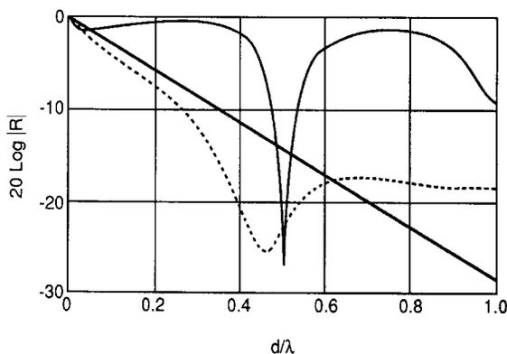
**Figure A4** Reflectivity of dominantly magnetic materials. Solid trace:  $|\mu_r| = 16$ ,  $|\epsilon_r| = 1$ ,  $\delta_\mu = 10^\circ$ ,  $\delta_\epsilon = 0^\circ$ ; dashed trace:  $|\mu_r| = 25$ ,  $|\epsilon_r| = 16$ ,  $\delta_\mu = 20^\circ$ ,  $\delta_\epsilon = 30^\circ$ ; diagonal trace:  $|\epsilon_r| = |\mu_r| = 4$ ,  $\delta_\epsilon = \delta_\mu = 15^\circ$  (from Knott, 1993, Fig. 8.13, p. 319).
