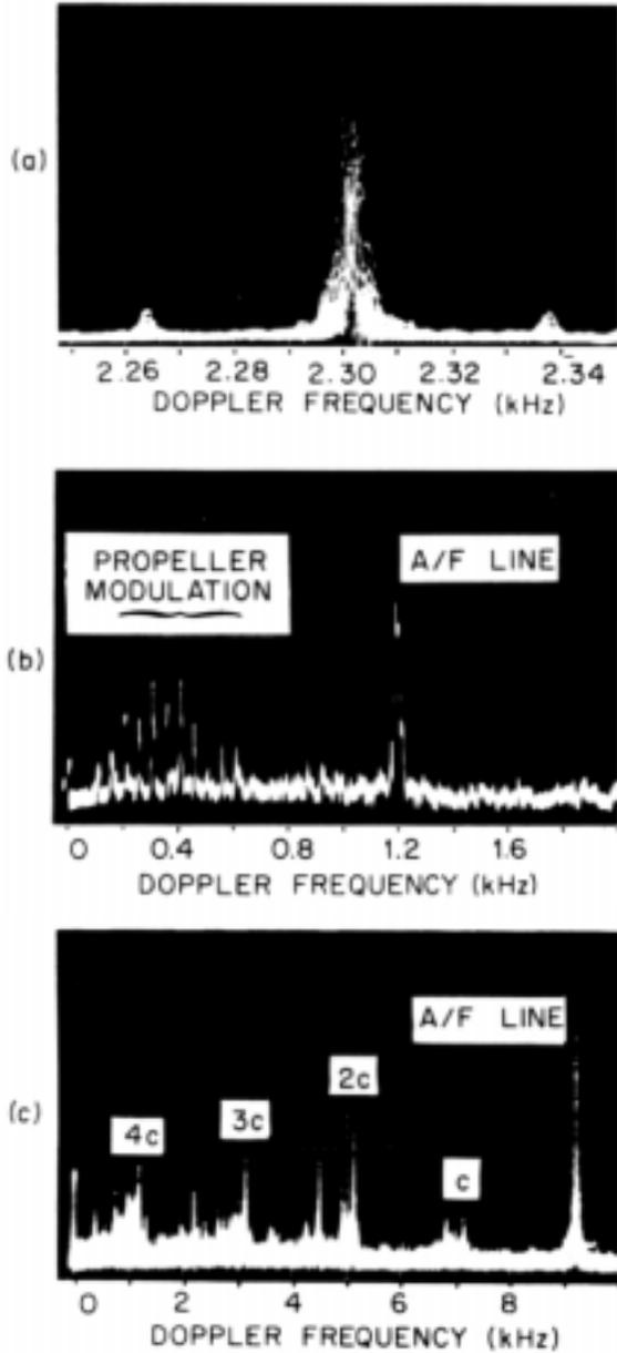
**Figure T5** Pulse-doppler spectrum measurements showing (a) an AM sideband pair caused by a conical-scan radar antenna; (b) FM modulation from propellers of a DC-7 aircraft; and (c) jet engine modulation at the compressor rotation rate and its harmonics (from Skolnik, 1970, Fig. 17, p. 28.22).
