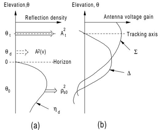
**Figure E11** Multipath reflection density and antenna pattern weighting functions in elevation coordinate. (a) Target and reflection components, (b) sum and difference antenna gains (after Barton, 1988, p. 520).
