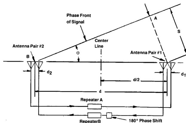
**Figure E3** Block diagram and wavefronts in cross-eye ECM (from Schleher, 1986, Fig. 3-7, p. 159).
