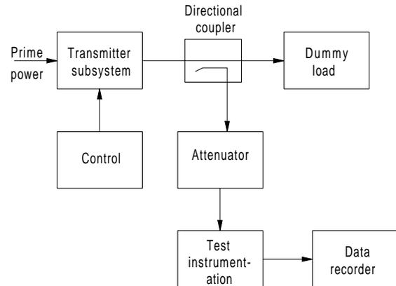
**Figure T15** Transmitter test configuration (after Barton, 1991, Fig. 13.5.3, p. 13.11).
