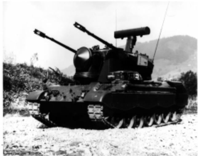
**Figure R29** Flakpanzer anti-aircraft tank system. The K<sub>a</sub>-band fire control tracker shares the forward antenna with a longer range X-band tracker, whose transmitter also serves the target acquisition radar at the rear of the turret.
