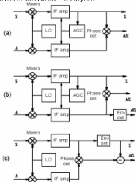
**Figure M21** Sum-and-difference angle discriminators: with (a) combined, and (b) separate formation of the magnitude and sign of the error signal, and (c) with normalization by the sum signal at video frequency (after Leonov, 1986, Fig. 1.5, p. 11).
