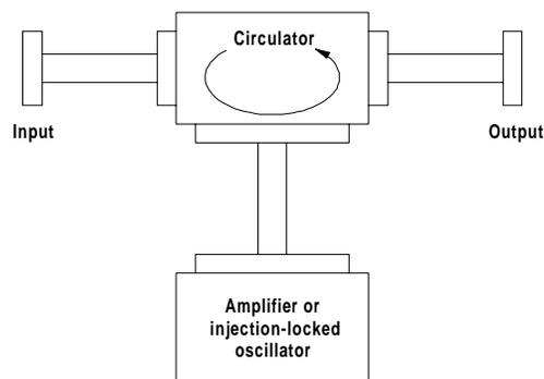
**Figure A38** Single-port amplifier (after Currie, 1987, Fig. 8.8, p. 406).
