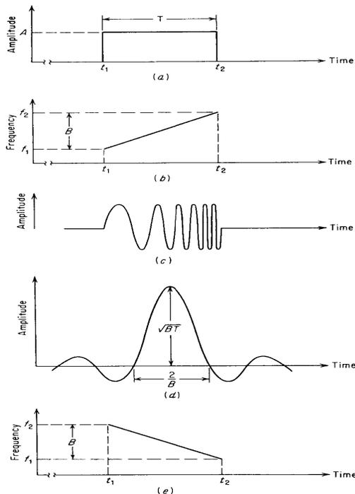
**Figure W11** Linear FM waveform and its compression: (a) transmitted waveform; (b) frequency of the transmitted waveform; (c) representation of the time waveform; (d) output of the pulse-compression filter; and (e) same as (b) but with decreasing frequency (from Skolnik, 1980, Fig. 11.15, p. 423, reprinted by permission of McGraw-Hill).
