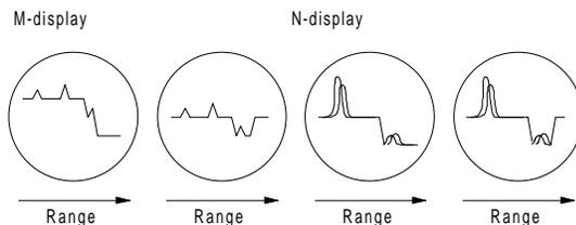
**Figure D53** M- and N-displays.
