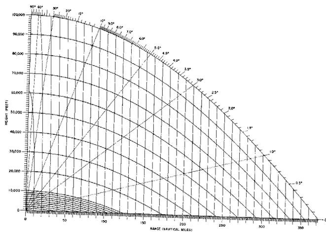
**Figure C16** Radar range-height-angle chart (from Skolnik, 1990, Fig. 2.18, p. 2.45)
