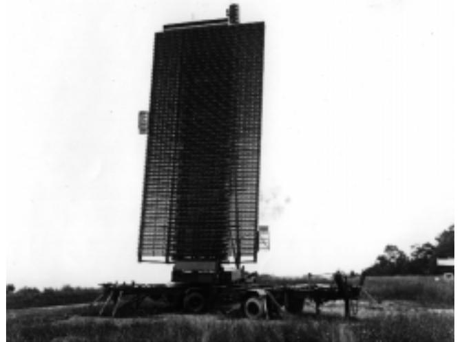
**Figure R64** AN/TPS-59 scanning-beam 3D radar. In this design, each row of elements has its own RF module, containing a power amplifier, a low-noise receiving amplifier, and a phase shifter (General Electric Co. photograph).
