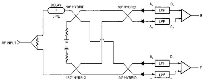
**Figure R94** A typical basic IFM receiver (from Vaccaro, 1993, Fig. 6.1, p. 128).
