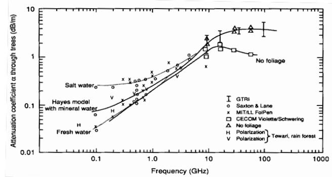
**Figure A98** Measured and calculated attenuation coefficient for trees vs. frequency (from Currie, 1992, Fig. 2.19, p. 81).
