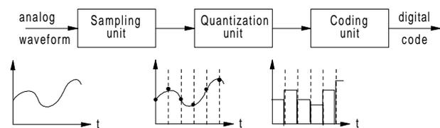
**Figure C40** Analog-to-digital converter.
