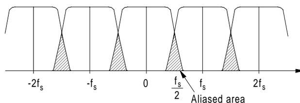
**Figure A21** Aliasing in the frequency domain (after Currie, 1989, Fig. 6.7, p. 183).
