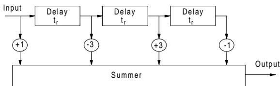
**Figure C3** Block diagram of four-pulse canceler.
