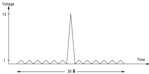
**Figure C32** Matched-filter output of Barker code of length 13.
