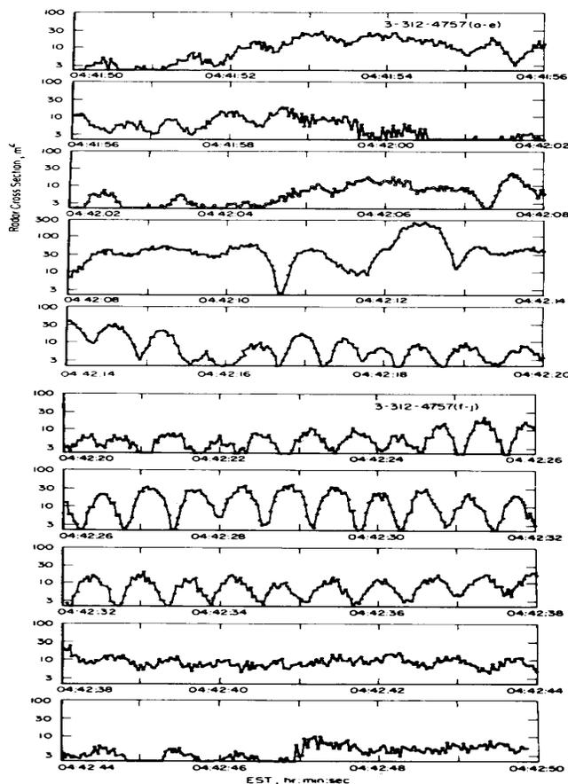
Figure R71 Plot of RCS in m<sup>2</sup> versus time for satellite, 1957 measured at 440 MHz (from Bhattacharyya, 1991, Fig. 1.18, p. 31).
