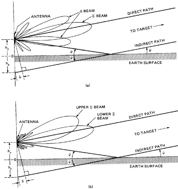
**Figure H2** Multipath effects on monopulse and squinted-beam height finders: (a) conventional  $\Sigma, \Delta$  monopulse, (b) squinted-beam low-angle technique (from Skolnik, 1990, Fig. 20.12, p. 20.37, reprinted by permission of McGraw-Hill).
