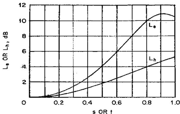
**Figure A60** Loss corrections for phase error in sectoral and pyramidal horns. The parameters  $s = b^2/(8\lambda l_e)$ , and  $t = a^2/(8\lambda l_h)$ , where  $l_e$  and  $l_h$  are the lengths of the horn flares (from Johnson, 1993, Fig. 15.8, p. 15.10, reprinted by permission of McGraw-Hill).
