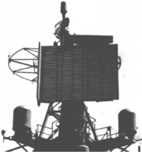
**Figure A82** AN/SPS-48 frequency-scanning 3D radar antenna.
