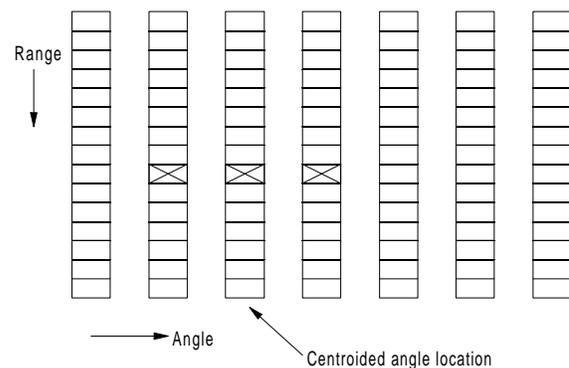
**Figure C13** Angle centroiding algorithm (after Morris, 1988, Fig. 13.11, p. 266).
