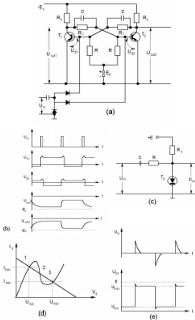
**Figure T28** Flip-flops: (a) symmetrical, (b) voltages of symmetrical flip-flop, (c) tunnel diode type, (d) characteristic of a tunnel diode, (e) voltages of tunnel-diode flip-flop (after Druzhinin, 1967, Fig. 6.26, page 240 and Fig. 6.30, page 243).
