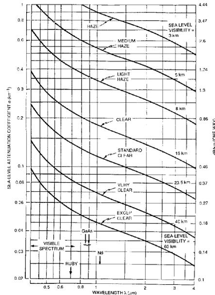
**Figure A100** Approximate variation of attenuation coefficients with laser wavelength, at sea level for various atmospheric conditions, excluding  $\text{H}_2\text{O}$  and  $\text{CO}_2$  components (from Jelalian, 1992, Fig. 2.3, p. 65).
