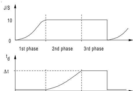
**Figure E5** Range gate pull-off operation.
