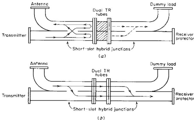
**Figure D57** Balanced duplexer using dual TR tubes and two short-slot hybrid junctions: (a) transmit condition (b) receive condition (from Skolnik, 1980, Fig. 9.6, p. 361, reprinted by permission of McGraw-Hill).
