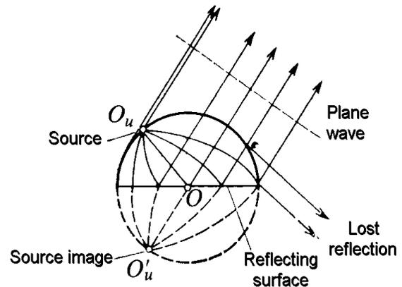
**Figure L5** Hemispheric Luneburg lens (from Leonov, 1986, Fig. 2.8, p. 20).
