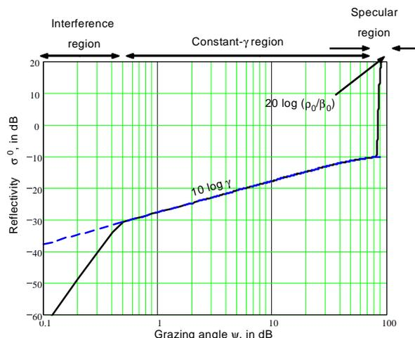
Figure C31 Typical surface clutter reflectivity vs. grazing angle.
