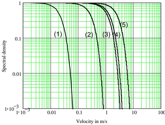
**Figure C30** Velocity spectra of five clutter types: in order of increasing spectral spread, (1) sparsely wooded hill, calm day,  $\sigma_v = 0.017$  m/s, (2) heavily wooded hills, wind 10 m/s,  $\sigma_v = 0.22$  m/s, (3) sea echo, windy day,  $\sigma_v = 0.89$  m/s, (4) chaff,  $\sigma_v = 1.06$  m/s, (5) rain clouds,  $\sigma_v = 2.0$  m/s (after Skolnik, 1980, Fig. 4.29, p. 132).
