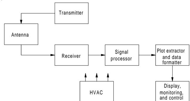
**Figure S29** Block diagram of typical radar by subsystems.
