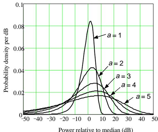
Figure C24 Weibull distribution, plotted as density in dB.
