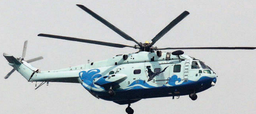
Above: Until a fixed-wing AEW platform is deployed, the Z-8YJ will play an important role as China's interim carrier-based AEW aircraft. First spotted in 2009, the 'Black Bat' features a retractable radar antenna attached to the rear ramp. The radar is reportedly a long-range multi-mode AESA type that can be lowered vertically to provide 360° coverage. via Chinese internet
