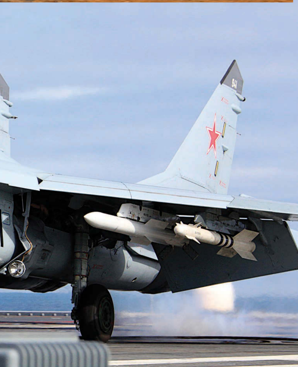
Below: Single-seat pre-production MiG-29K 'Bort 941' conducts deck trials in July 2012. The two-seat and single-seat versions feature exactly the same fuselage and canopy, but the latter has a fuel tank in place of a rear seat. Images by RAC MiG unless credited otherwise
