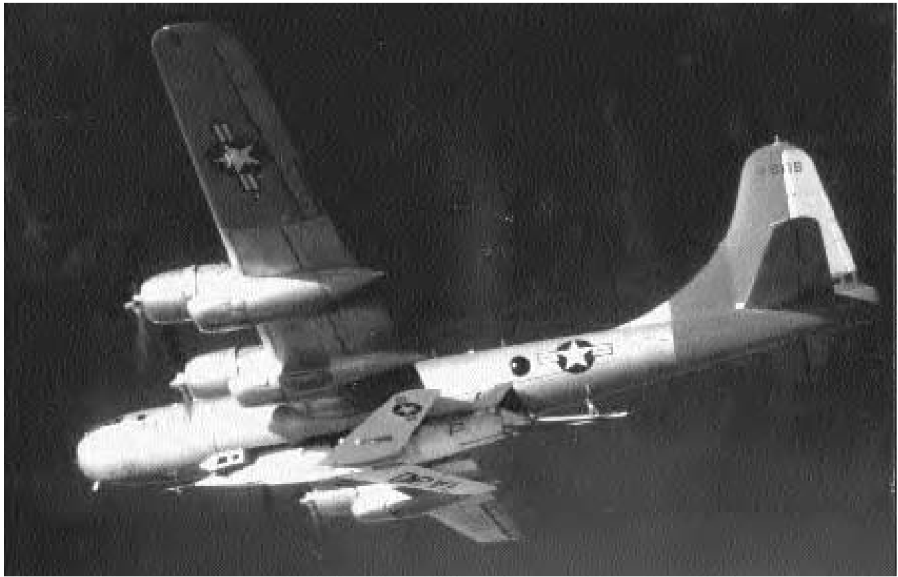
The Bell X-2 suspended below a Boeing B-50D carrier plane. (Walter J. Boyne)
