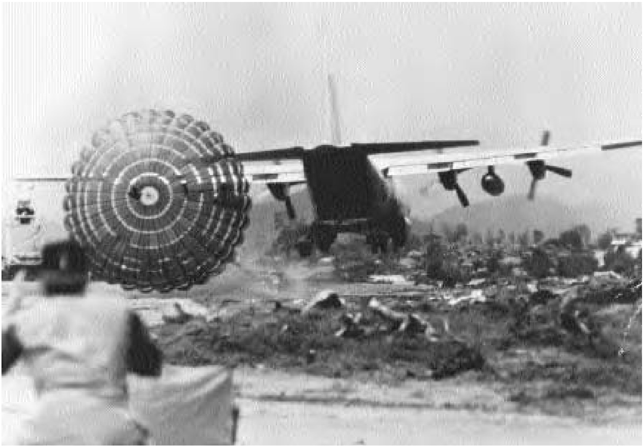
LAPES stands for Low Altitude Parachute Extraction System, shown here in combat. (U.S. Air Force)
