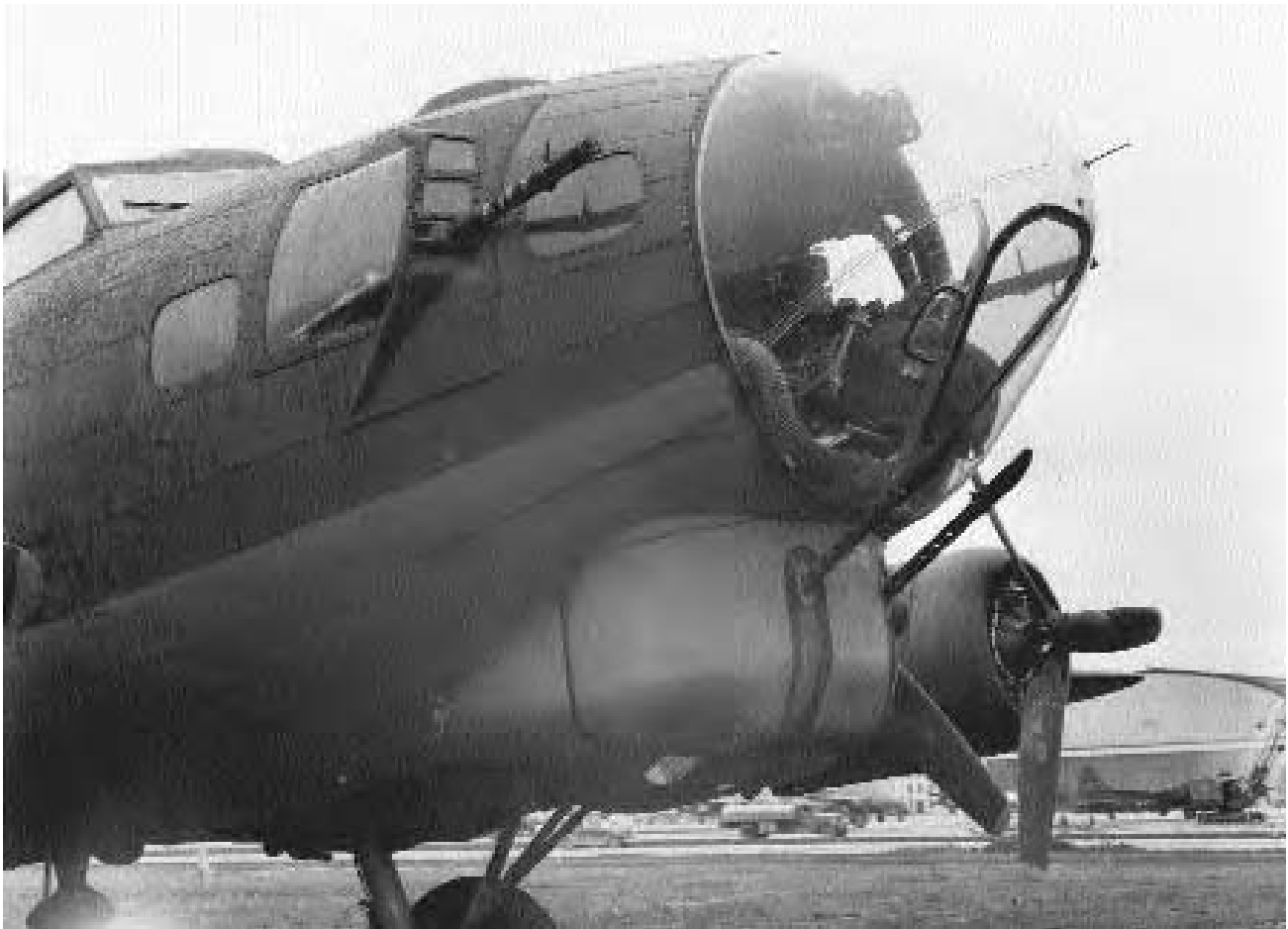
The demands of air combat caused many modifications to be made to Boeing's B-17, and among the most important of these was defensive firepower. This B-17G packed a powerful forward-firing turret to offset German frontal attacks. (U.S. Air Force)
