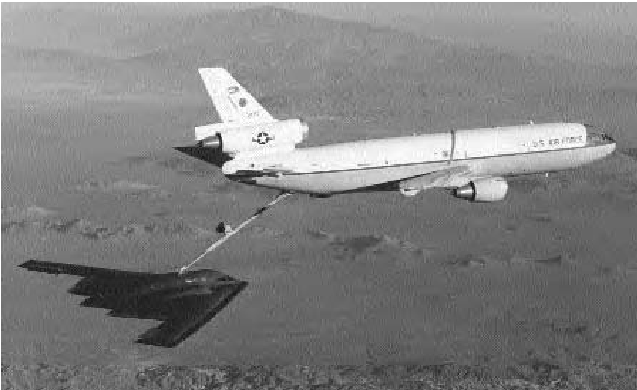
The Boeing KC-10 tanker is employed for many specialized refueling jobs, including taking care of the Northrop B-2A. (U.S. Air Force)
