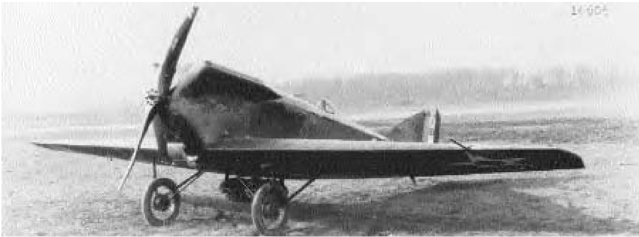
Designed by Alfred Verville and built in the Sperry plant, the Verville Sperry was years ahead of its time with its low cantilever wing and retractable landing gear. Inadequate testing kept it from entering service. (U.S. Air Force)
