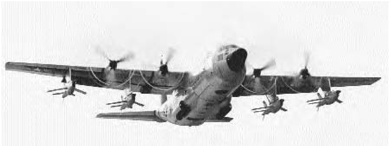
The name Ryan always meant quality and never more so than with the Firebee drones being carried on the versatile Lockheed C-130 transport. (U.S. Air Force)
