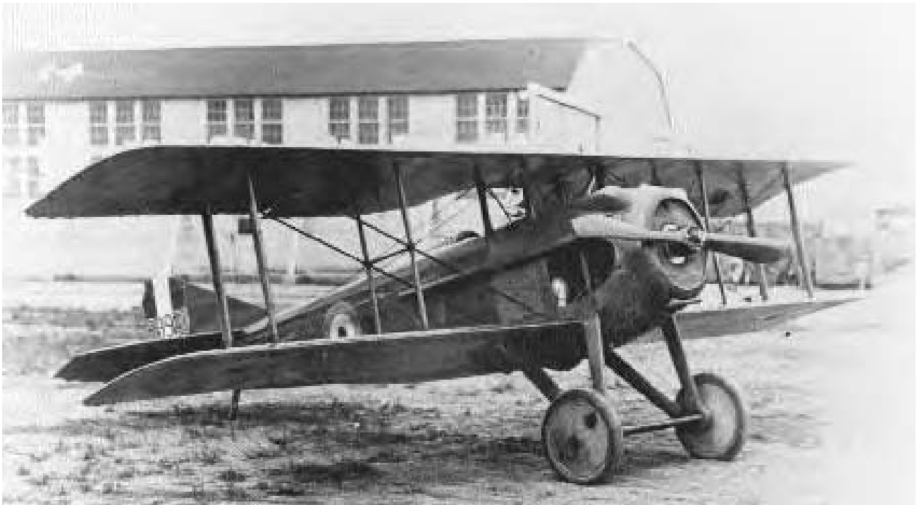
The SPAD VII was a welcome replacement for the earlier Nieuport series of fighters, for while the Nieuports suffered from structural weakness, the SPAD was strongly built and capable of a good turn of speed. (U.S. Air Force)
