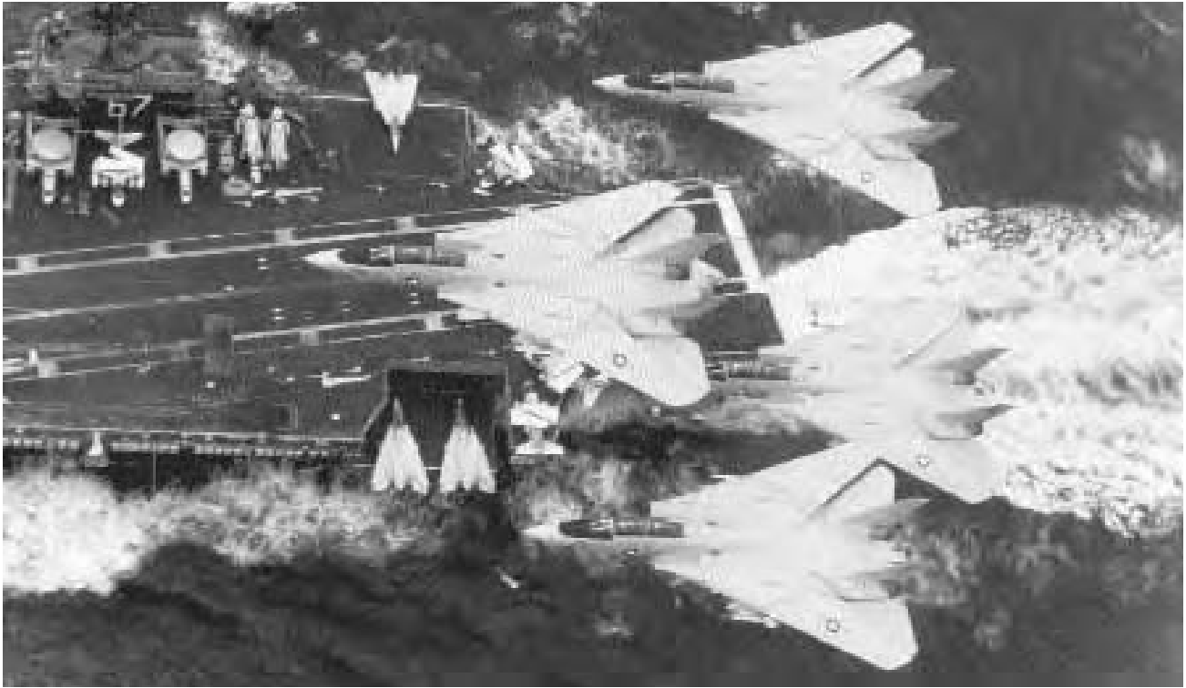
The swept-back wings of these Grumman F-14 Tomcats reveal that they are making a high-speed pass. Complex and not easy to fly, the Tomcat gained its greatest public acclaim in the film Top Gun, but it was already highly regarded by professionals. (U.S. Navy)
