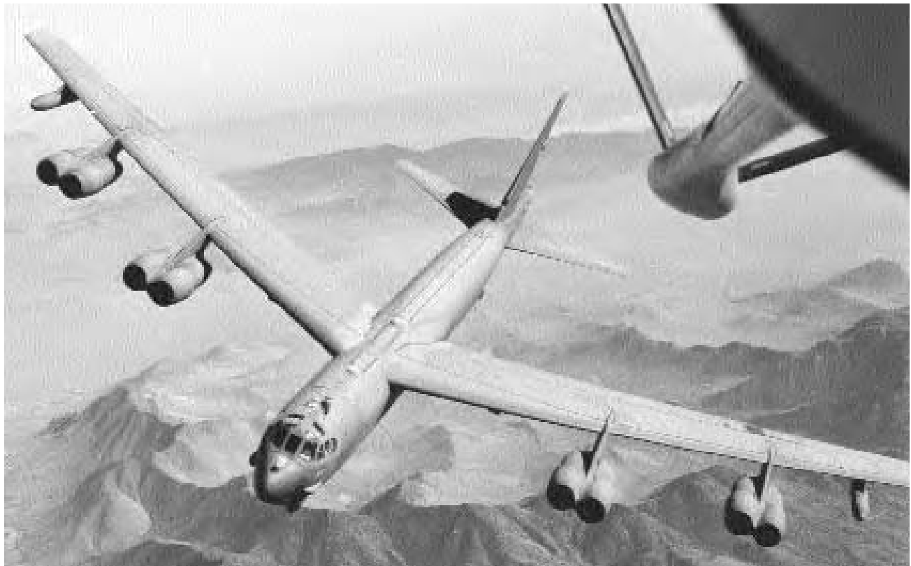
This photo, taken from the boom operator's position of a Boeing KC-135, represents a routine event that nonetheless takes tremendous skill: the refueling of a Boeing B-52 bomber. (U.S. Air Force)
