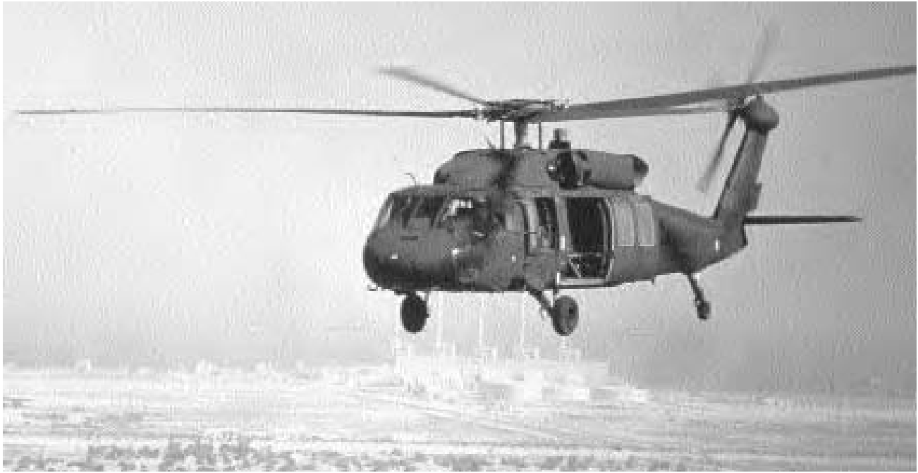
Developed in 1974 as result of the Utility Tactical Transport Aircraft System (UTTAS) program, the Sikorsky H-60 offers dramatic improvements in troop capacity and cargo lift capability over earlier helicopters. (Walter J. Boyne)
