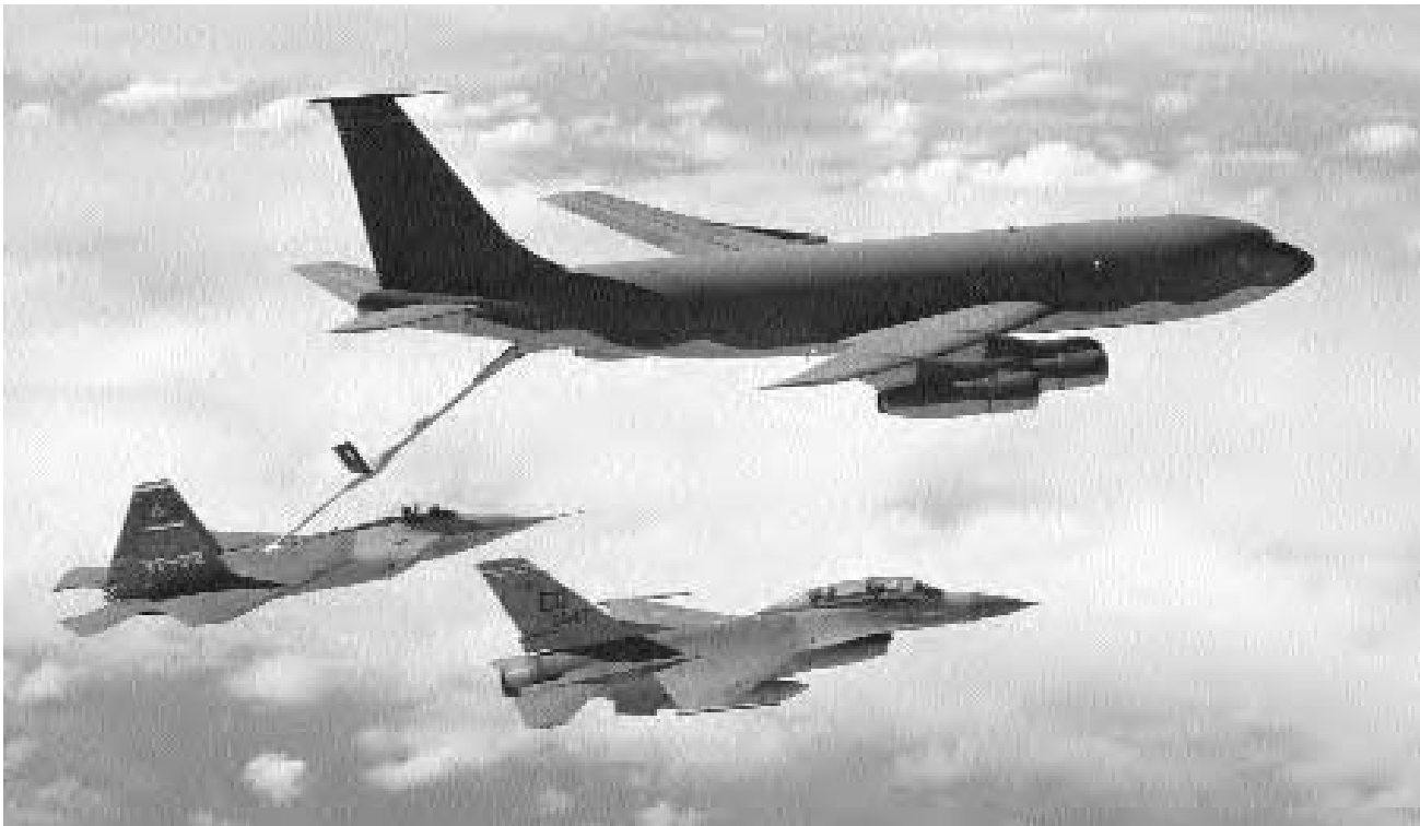
The different configurations of aircraft require that much inflight refueling testing be done to ensure compatibility. A Boeing KC-135 refuels a YF-22 while an F-16 flies chase. (U.S. Air Force)
