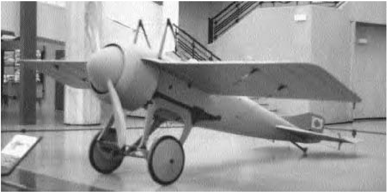
The simple, clean lines of the Deperdussin racer were the key to its high 127 mph speed in 1913. (Walter J. Boyne)
