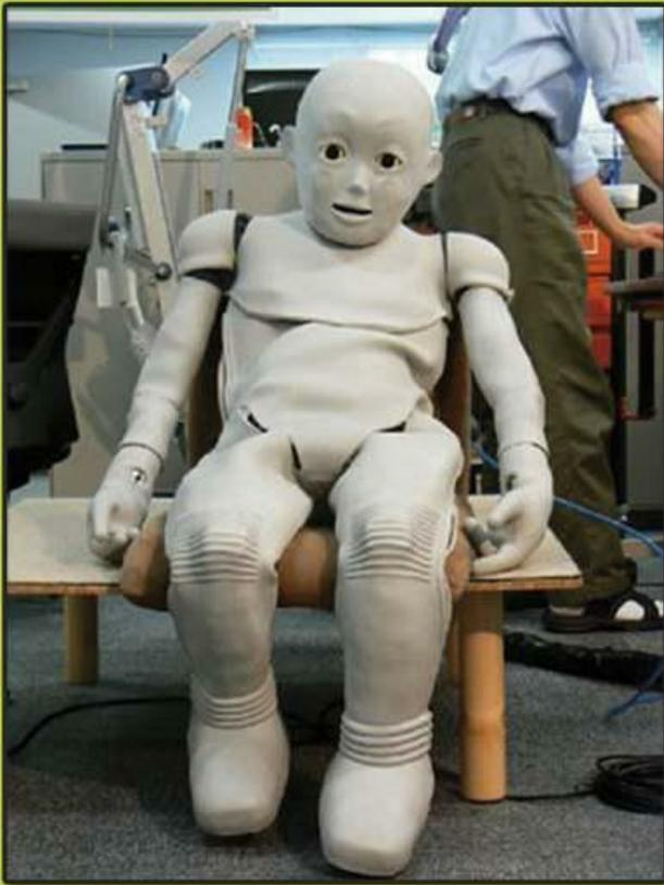
**The CB2 (the “Child Robot”) is another project developed by the researchers at Osaka University. CB2 has the physical and intellectual abilities of a 2-year old. It was built with cameras for sight, microphone, and tactile sensors to simulate a sense of touch and feeling. “One day,” says Professor Ishiguro, “they will live among us. Then you’d have to ask me, “Are you human?”**
