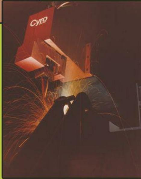
**Close up of the Advanced Robotic's Cyro 2000® rectilinear arc welding robot. The Cyro 2000 is the largest arc welding robot in the world.**
