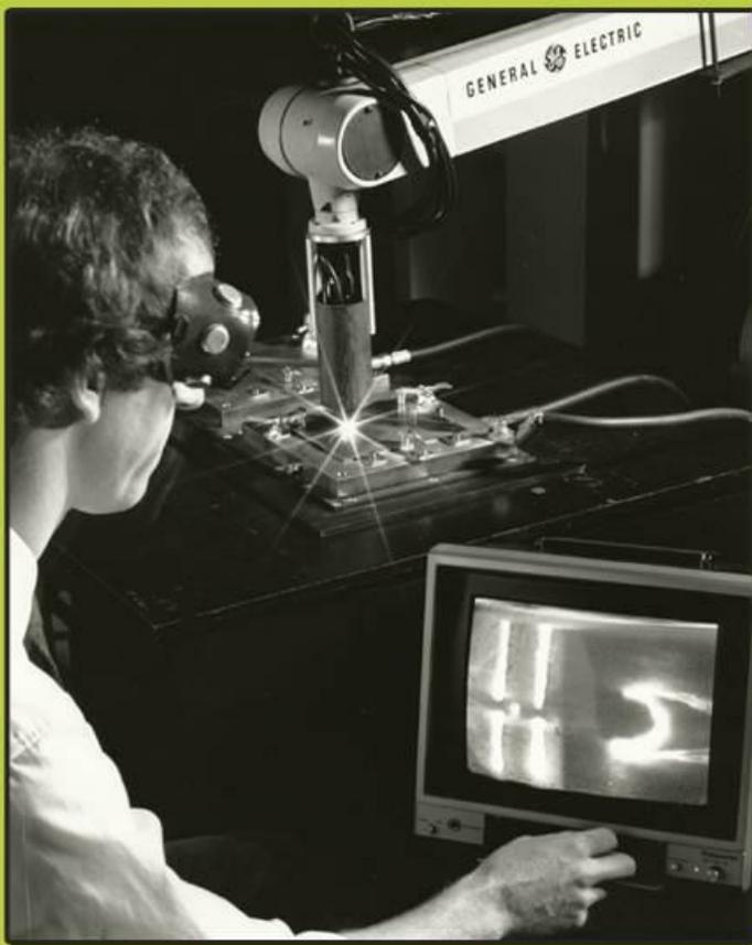
**This General Electric robot has a sensor system that brings the powers of sight and intelligence to welding robots. The advanced vision and control system enables a welding robot to steer itself along irregularly shaped joints, continually observing the joint and weld “puddle” and making adjustments as it travels along.**
