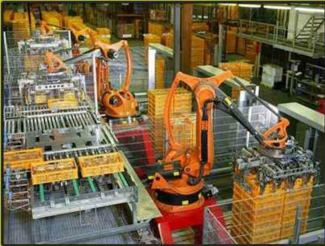
**Modern robot packers at work packing bread.**
