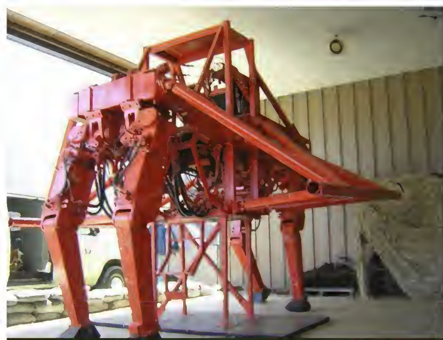
In 1966, General Electric was commissioned by the U.S. Army to design this walking humanoid. Impractical, it gulped down 50 gallons of oil per minute.
