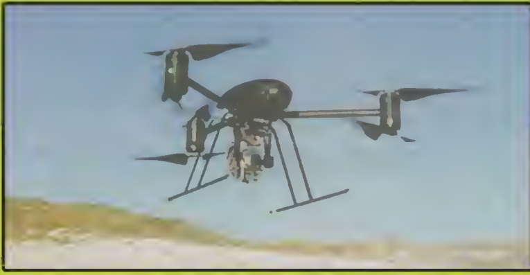
The Draganflyer X6 drone during a test flight in Mesa County, Colorado. Only 36 inches long, it weighs two pounds.
