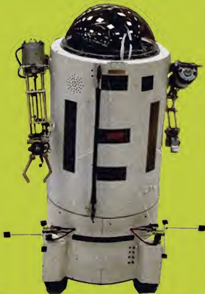
H.E.N.R.Y., built by Bruce C. Taylor, uses bumpers to stay clear of obstacles. This robot possesses a 128-word vocabulary and has two workable arms. (theoldrobots.com)
