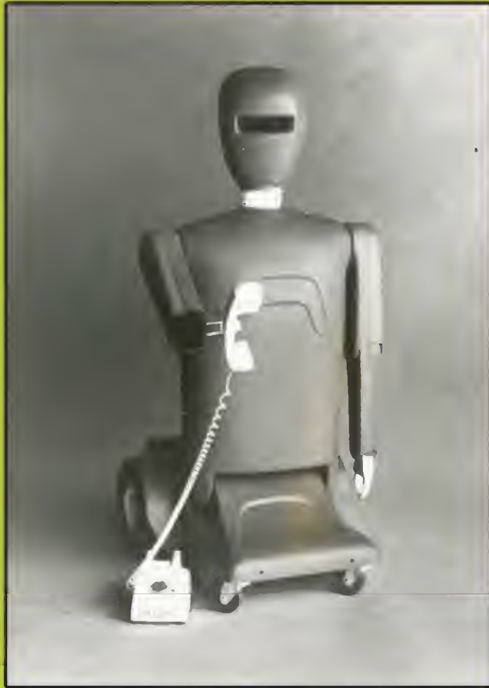
Marvin was “born” in 1985. His father was Iowa Precision Robotics, Ltd. Marvin moves on his wheels, speaks 500 words, moves his head and is controlled by computer.
