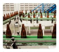
In mass production, most process are automated. In this factory, bottles are transported from one machine to another
