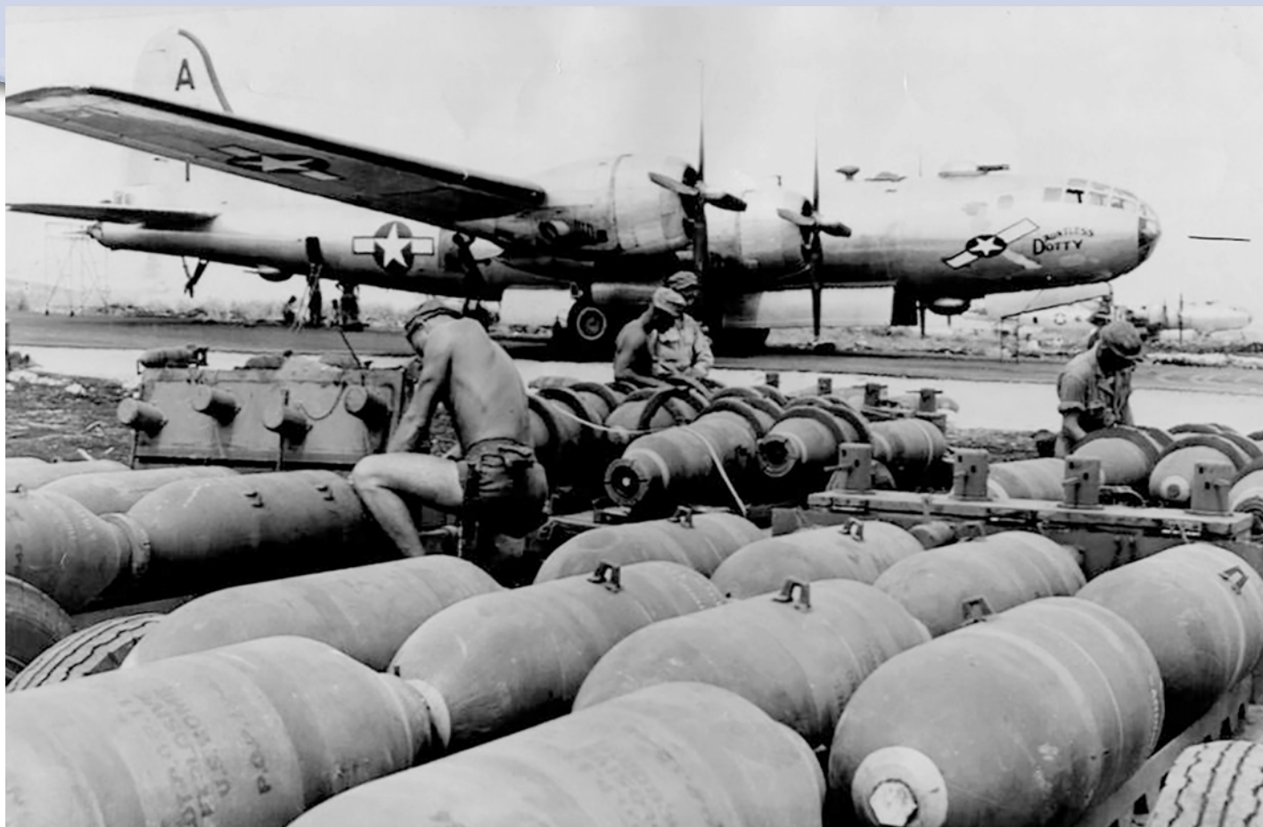
Nearly 340 B-29 Superfortresses of the U.S. Air Force participated in the Operation Meetinghouse firebombing of Tokyo. It has been calculated that 1,665 tons of bombs were dropped on Tokyo in the attack. Most were 500-pound E-46 cluster bombs (above) which released 38 napalm-carrying M-69 incendiary bomblets that hit the ground, then exploded, ejecting globs of fiery napalm on anything nearby. More than 100,000 Japanese civilians were killed.
