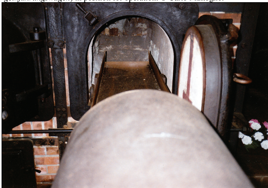
Document 41: Crematorium of Buchenwald. Topf triple-muffle coke-fired oven. Central muffle. Corpse introduction cart with loading stretcher inside the muffle. © Carlo Mattogno.
