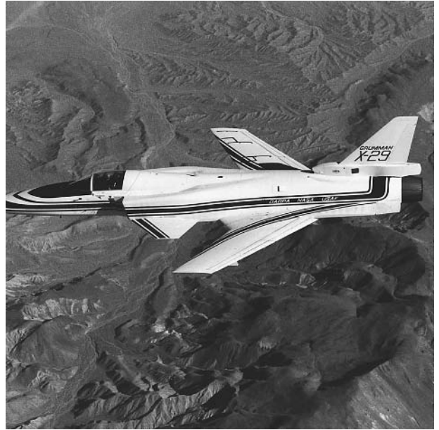
In a joint research project, the Defense Advanced Research Projects Agency, NASA, and the U.S. Air Force used a Grumman X-29 with a forward-swept wing in fighter research during the 1980's and 1990's. ©MUSEUM OF FLIGHT/CORBIS.
