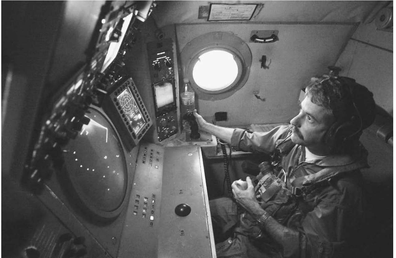
A U.S. Navy aviation systems warfare operator searches for and tracks surface contacts using radar and the Infrared Detection System of his P-3 Orion patrol aircraft during a routine flight in support of Operation Enduring Freedom in October 2001. AP/WIDE WORLD PHOTOS.
