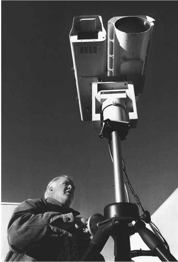
An electronics technician for the U.S. Border Patrol uses a crank to manually turn two surveillance cameras, a thermo imager, right, and a daytime camera, left. AP/WIDE WORLD PHOTOS.
