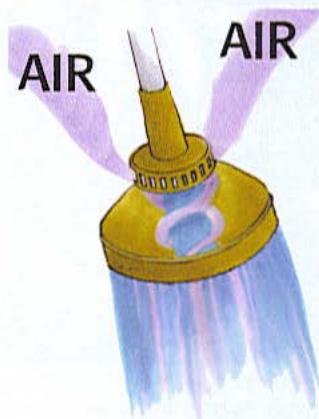
A water wand with a breaker head mixes air with irrigation water just before applying.
