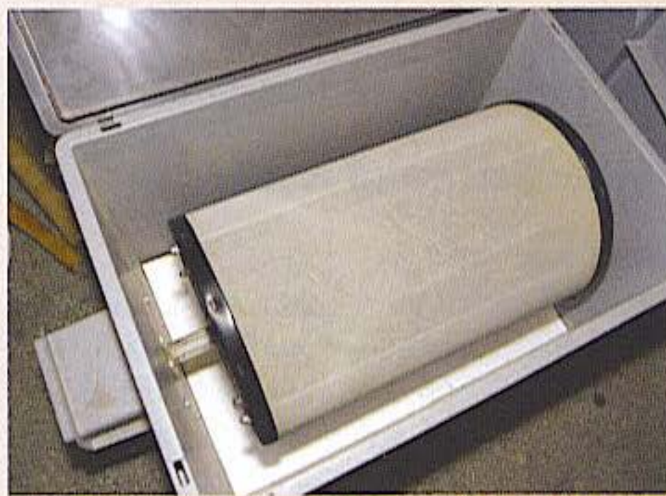
Put the lid back on the drum, and set it back in the Pollinator. Close the top of the Pollinator, and turn it on for the first turning period.
