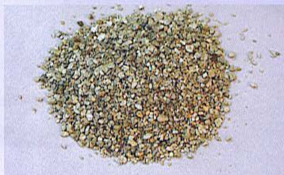
Vermiculite holds a lot of nutrient solution.
