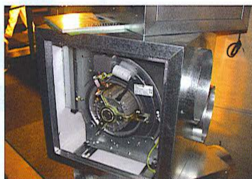
Here is an example of a heavy-duty extractor fan from a Dutch grow room.
