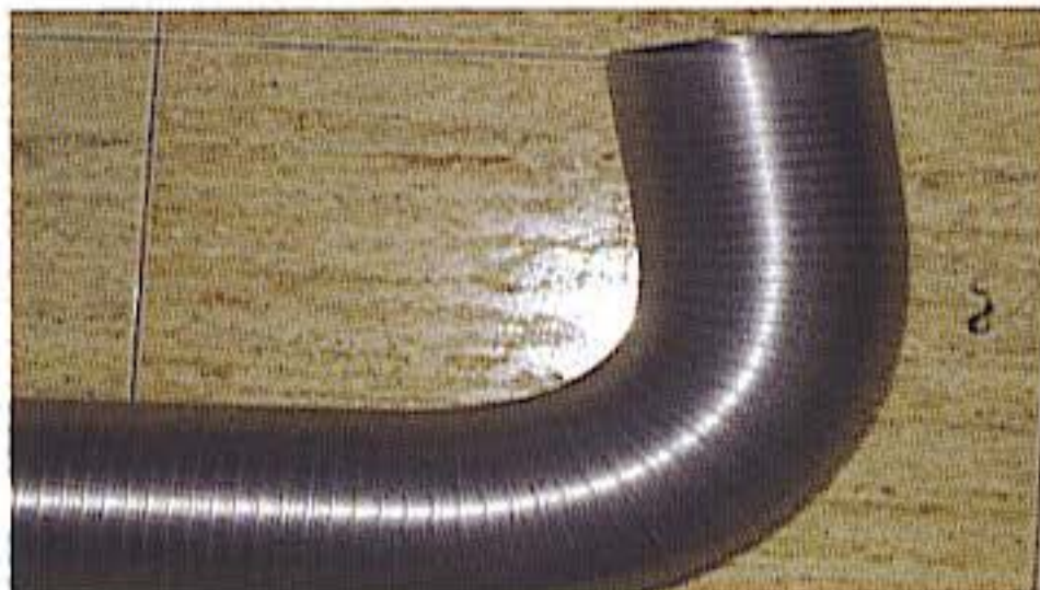
Ninety degree curve cuts up to 60 percent of air transmission.
