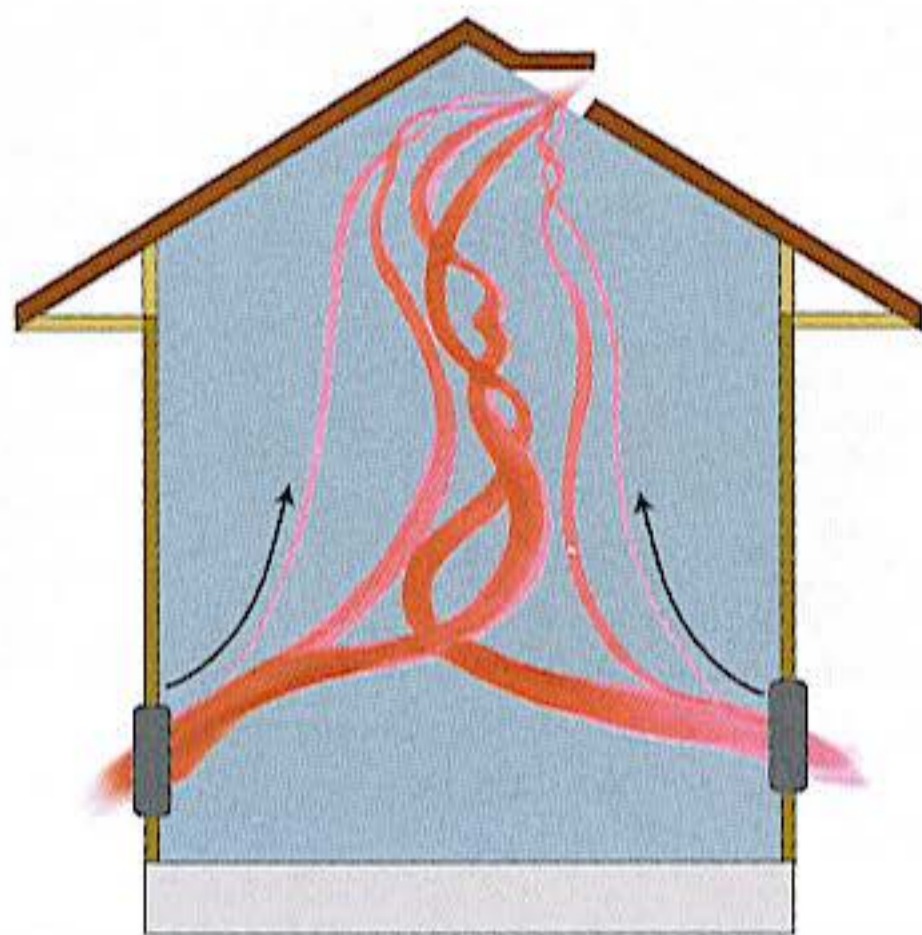
Hot air flows upward naturally. Always design grow rooms and greenhouses to take advantage of this principle.
