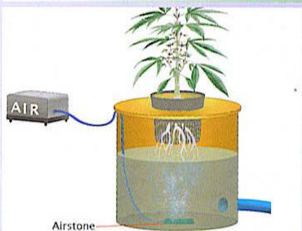
Cutaway of the inside of a DWC garden
