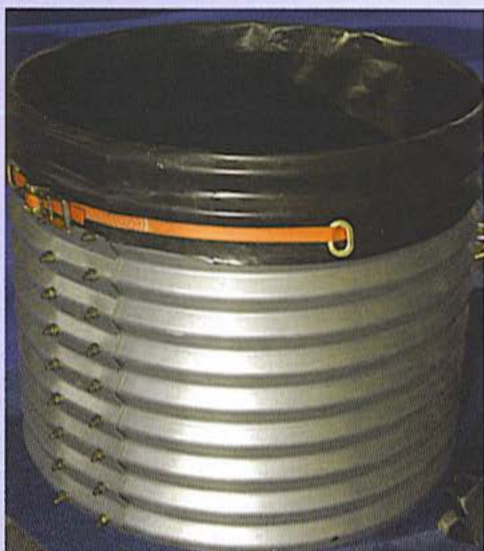
This innovative reservoir was made by lining a large galvanized pipe with heavy-duty plastic.
