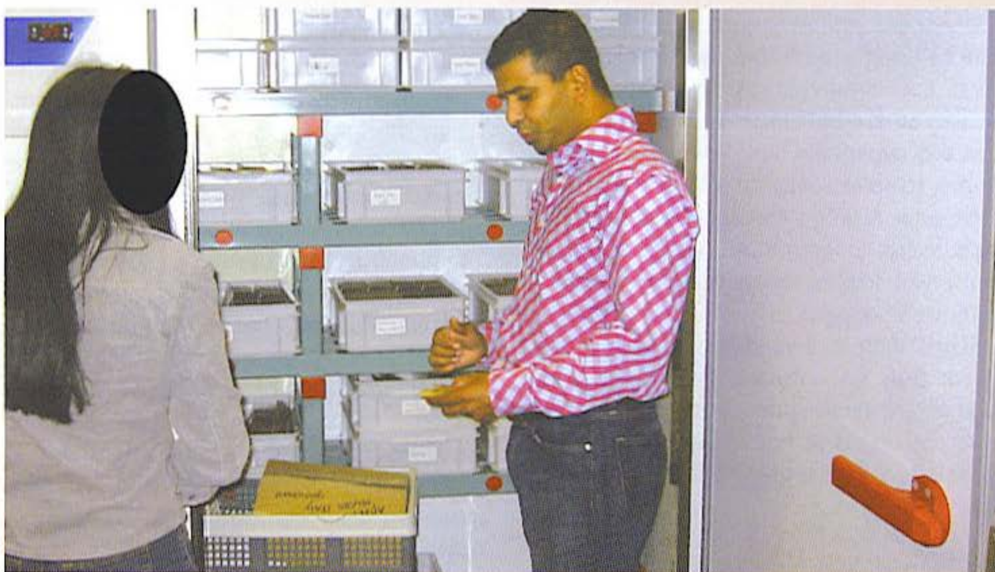
Boy Ramsahai, owner of High Quality Seeds and Black Label Seeds, shows off his high-tech refrigerator for seed storage. The refrigerator keeps humidity levels below five percent to ensure safe long-term storage.
