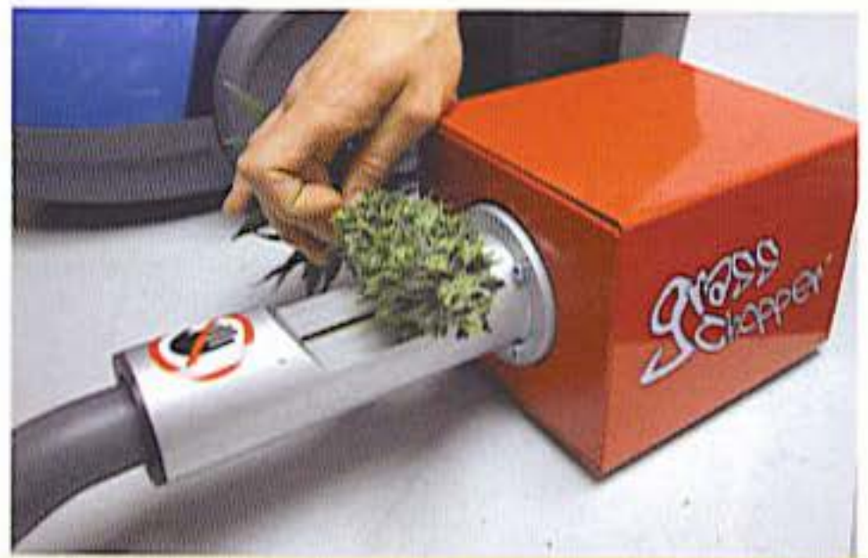
The Grass Chopper is one of the many new medium-sized bud trimmers that feature vacuum leaf removal.
