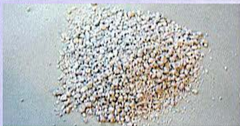
Perlite is sand or volcanic glass expanded by heat. See Chapter Ten for more information.
