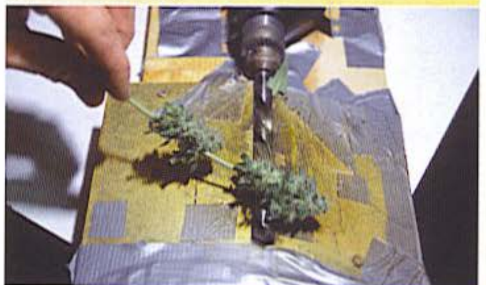
This ingenious grower made a bud trimmer by duct taping a couple of pieces of metal and a drill to a workbench.
