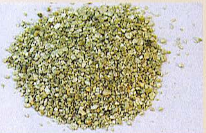
Vermiculite is lightweight and absorbent.
