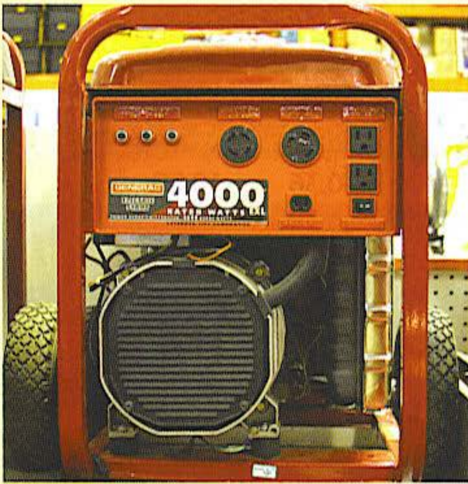
This generator produces 4000 watts at full capacity.
