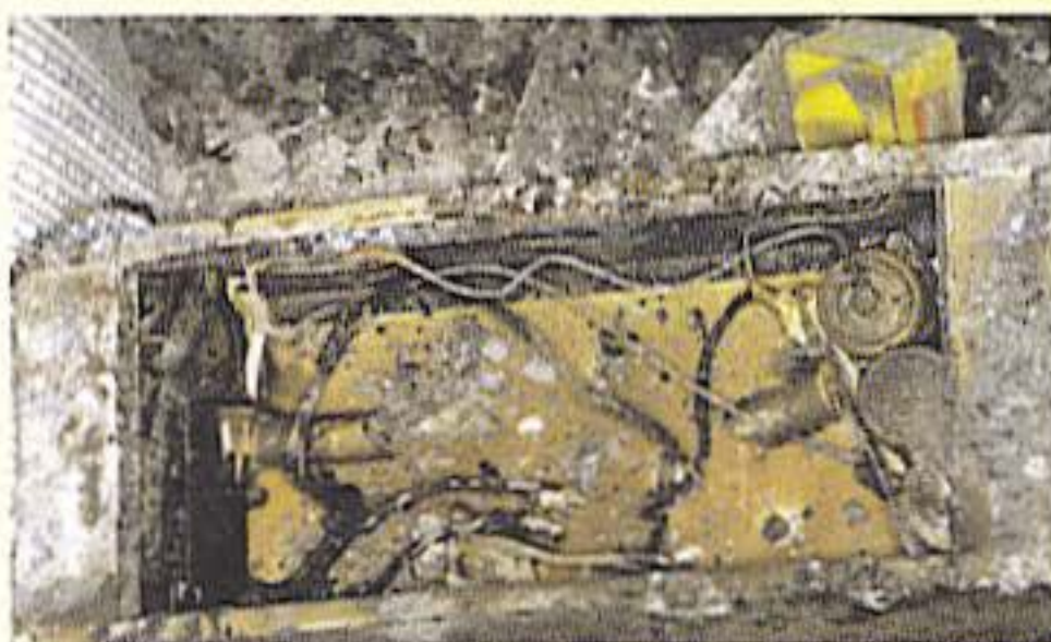
This grower lost the crop! He also almost lost his life! Pay attention to electrical connections, ampere ratings for wire, breaker switches, and connectors.
