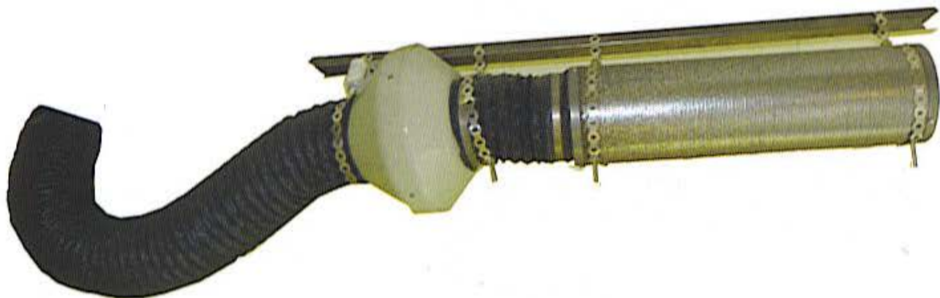
Here is a charcoal filter without the outer dust filter. The in-line fan adds extra suction to pull and push air through flexible ducting before it meets the extraction fan at the end of the duct.
