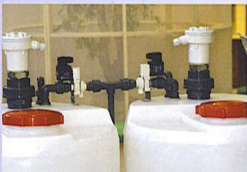
A two-part nutrient solution is mixed before application. Each reservoir holds one part of the solution.
