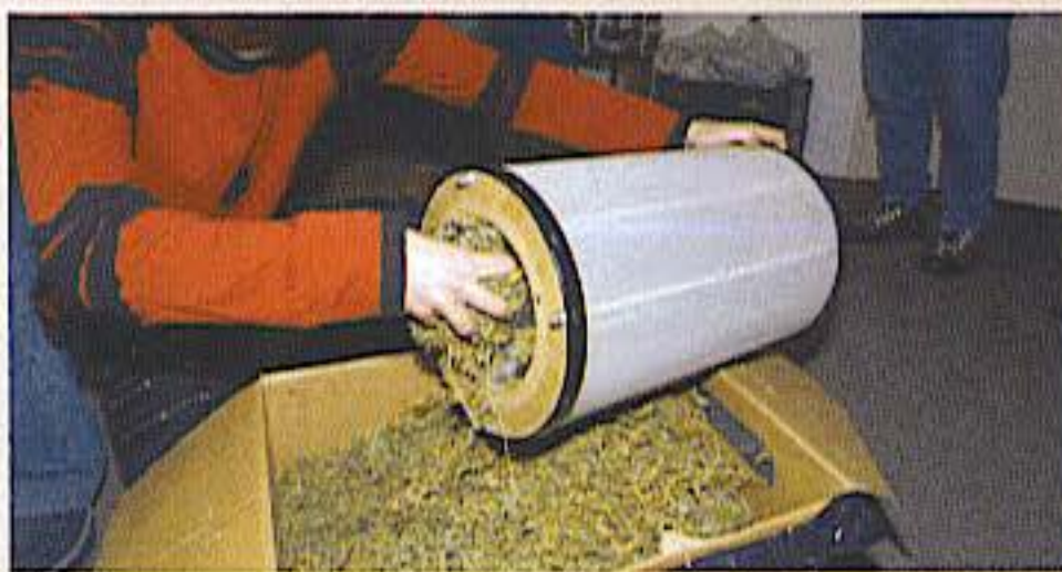
Remove the magnetic lid from the drum, and add small leaves and buds. Do not put any sharp sticks or objects into the drum, because they could damage it.
