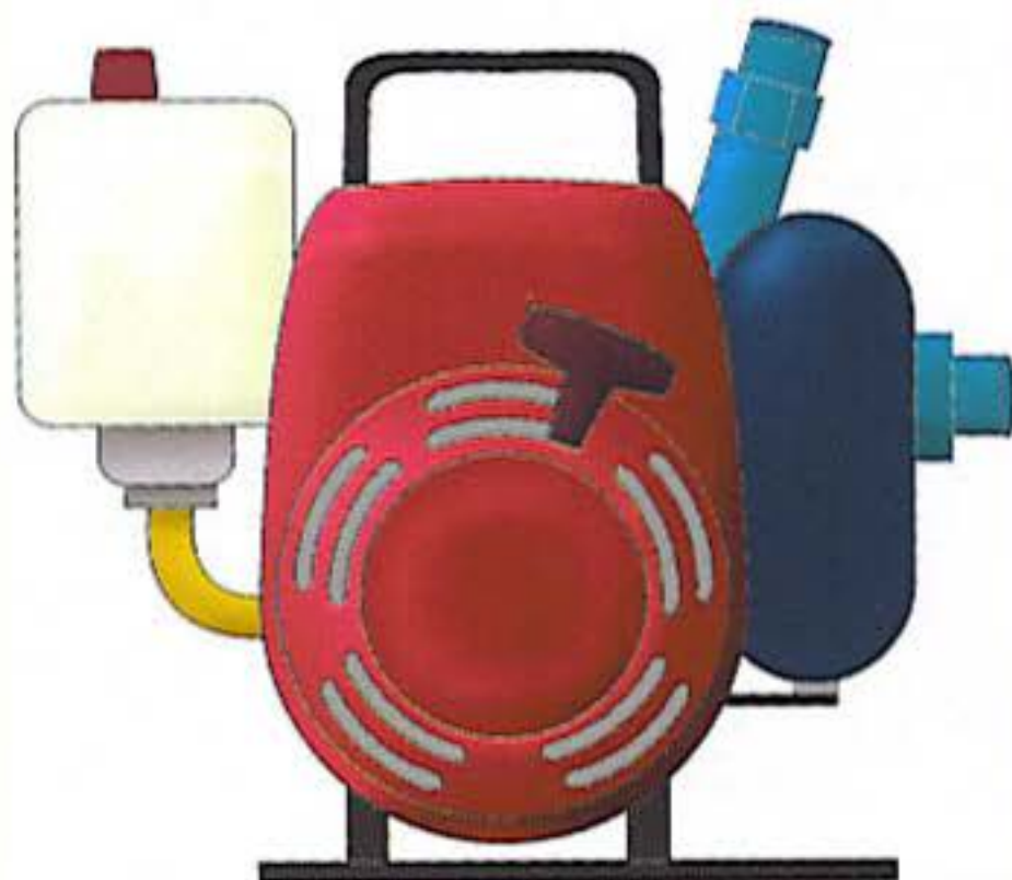
A gasoline-powered pump moves much water uphill, but they are noisy!
