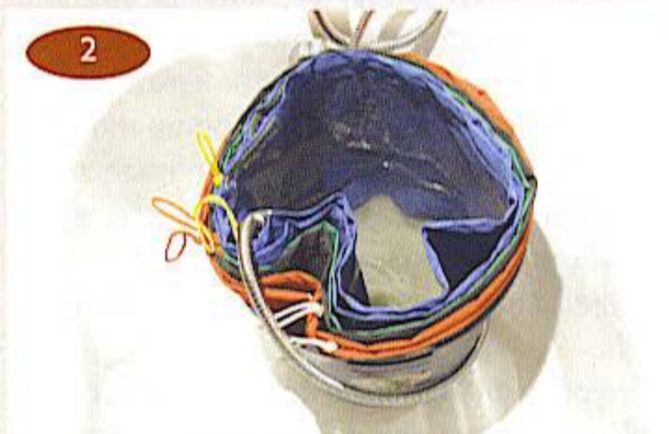
Fill the bags at least halfway up and above the level of the screens. The screens must be covered with water before introducing plant matter.
