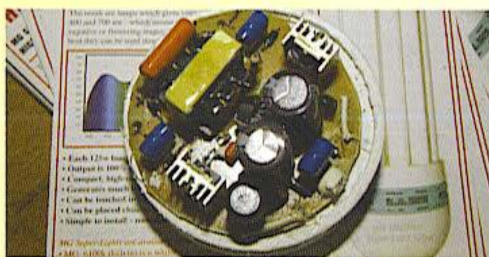
The inside of an electronic CFL ballast is compact and creates very little heat.
