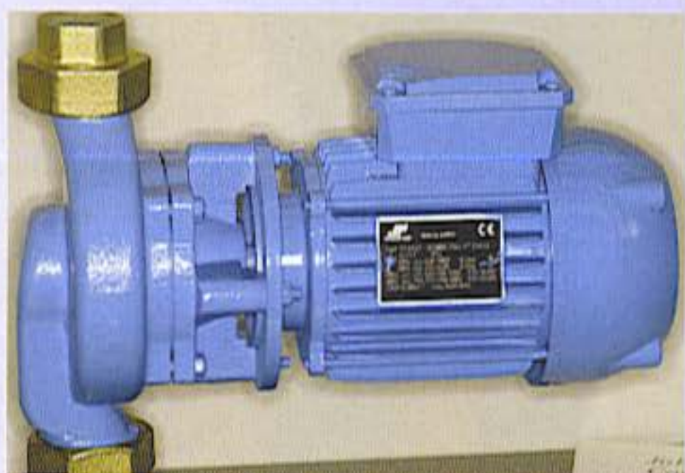
Large non-submersible pumps quickly and efficiently move considerable volumes of nutrient solution.
