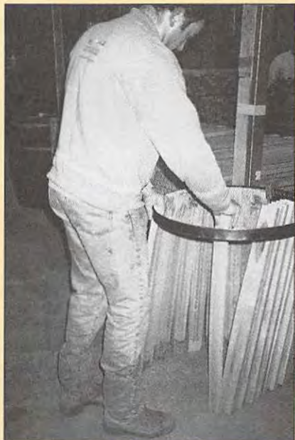
Barrel making is practiced today in much the same way it has been for centuries. The oak is hand split (with a little mechanical help) along the grain (left). Staves are carefully placed into position (right) using nothing but an iron hoop and a lot of skill.
