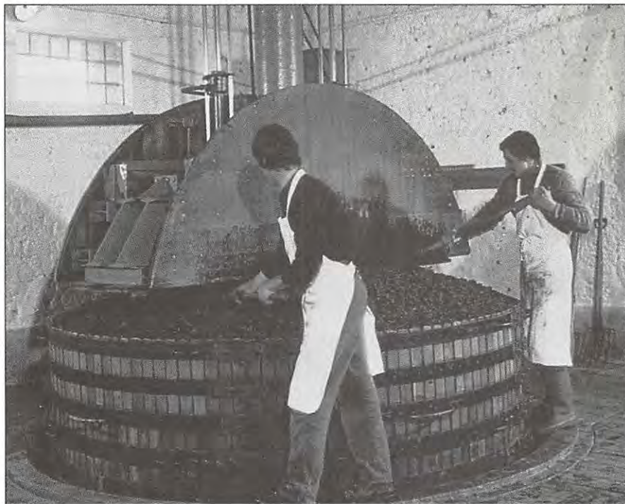
Wooden basket presses were formerly the norm in Champagne. Most of these presses were not ideal since grapes in them could be easily bruised and abraded, leading to coarse wine. Modern pneumatic presses are much more gentle.
