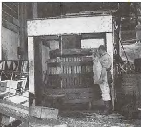
Computer-operated pneumatic bladder presses (left) are now common sights in modern wineries, though in the early part of the twentieth century, most wines were still made in rudimentary basket presses (above).
