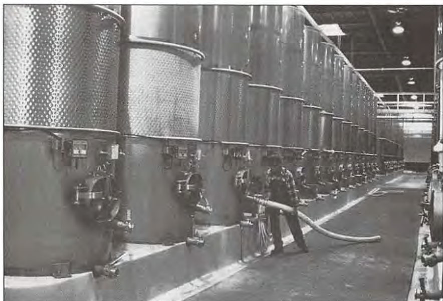
The introduction of temperature-controlled stainless steel tanks revolutionized the wine business by giving winemakers far greater control over the fermentation. White wines, in particular, benefited from the new tanks, which, by keeping the wine cool, better preserve delicate aromas and flavors.
