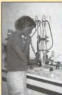
Wineries regularly test for the amount of sulfites in a wine; these are compounds that occur naturally as a result of fermentation.
