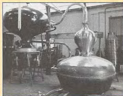
Small copper pot stills called alambics charentais are traditional for distilling Cognac.
