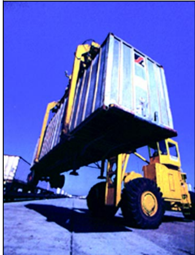
Side-loader at CSX Sea-Land Intermodal Terminal
