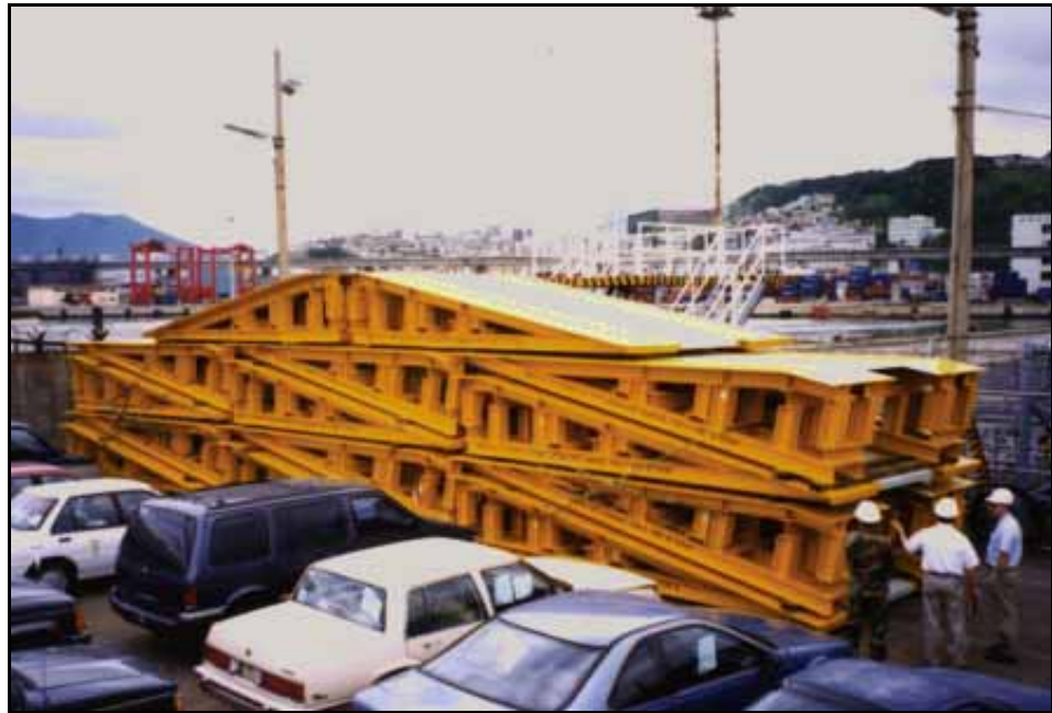
Portable Steel End Ramps at Pier 8
