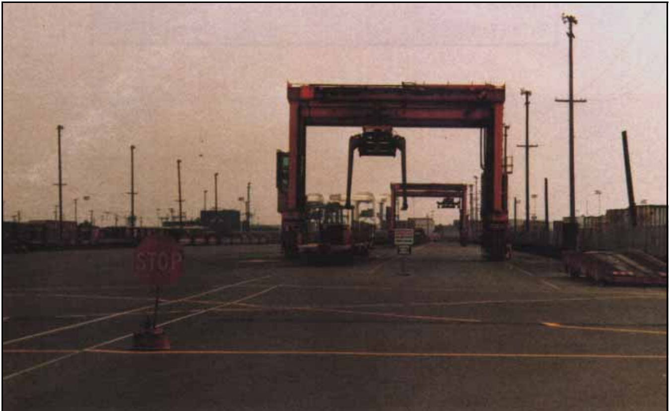
Southern Pacific Intermodal Yard Straddle Crane (Transtainer)
