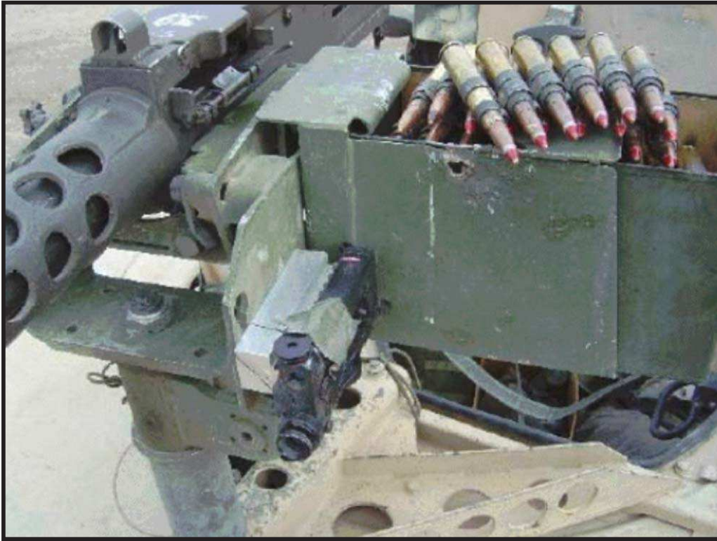
Figure 1-XII-2: PEQ-2 on fabricated mount (note tracer starter belt)
