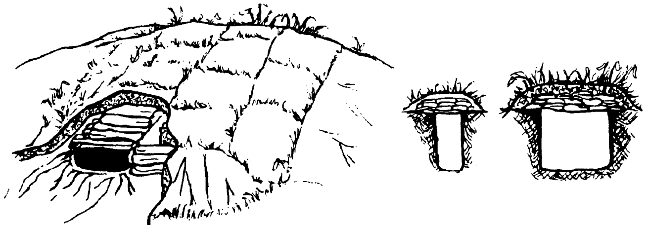
Figure 4-6. Sandbags protected with sod and earth cover.
