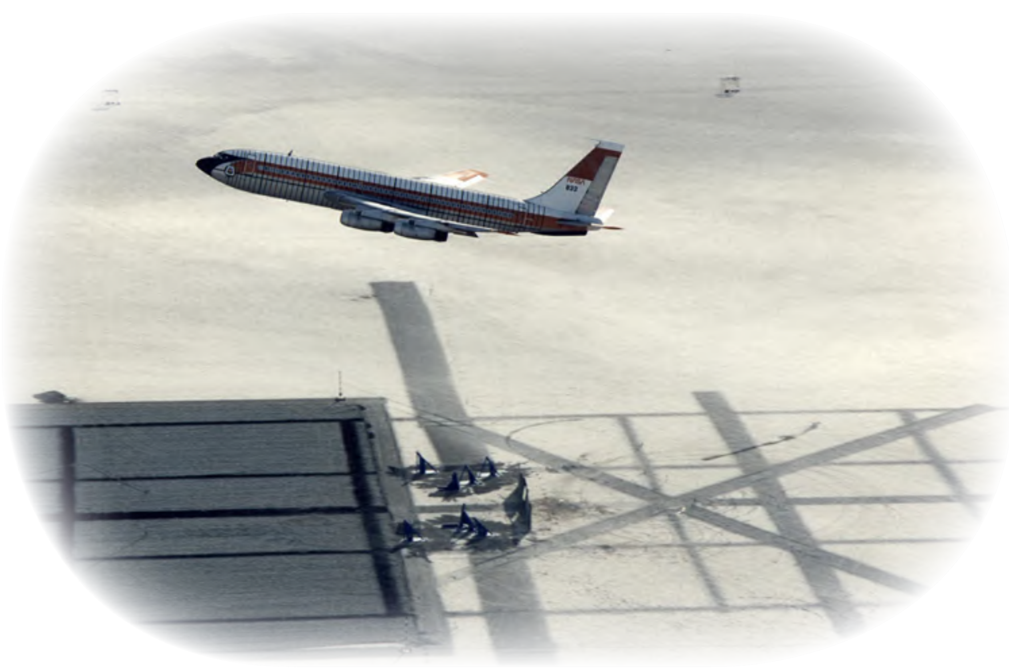
Boeing 720 - In this photograph (above) the B-720 is seen making a practice close approach over the prepared impact site. The wing openers, designed to tear open the wings and spill the fuel, are clearly seen on the ground just at the start of the bed of rocks.
