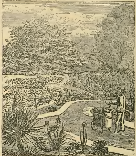
FIG. 50.—Read's Garden Engine.
