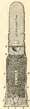
FIG. 4.—1, sheet brass; 2, copper; 3, wrought iron; 4, paper; 6, mill-board; 7, bees-wax.
