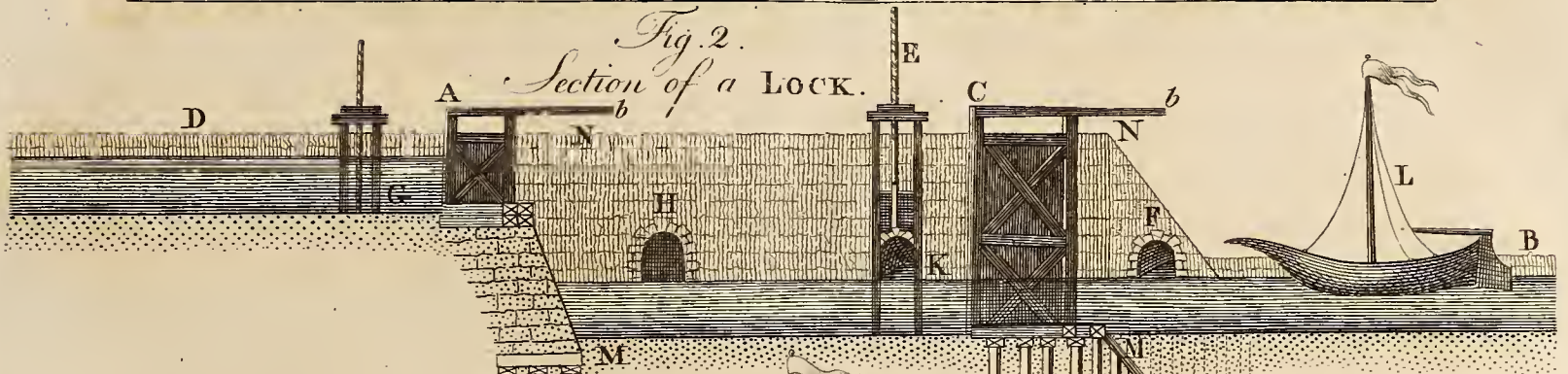
Fig. 3. Section of a LOCK full of Water.
