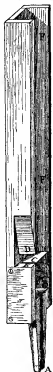
From V. Mahillon, Éléments d'acoustique , by permission of C. Mahillon. FIG. 1.—Diagram of a flue-pipe.
