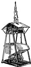
FIG. 17.—Light steel safety mining cage and car for gold and silver mines. Wellman-Seaver-Morgan Co., Cleveland, Ohio, makers.
