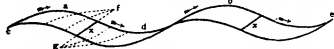
FIG. 13.—Wave track made by the wing in progressive flight. a, b , Crests of the wave; c, d, e , up strokes; x, x , down strokes; f , point corresponding to the anterior margin of the wing, and forming a centre for the downward rotation of the wing ( a, g ); g , point corresponding to the posterior margin of the wing, and forming a centre for the upward rotation of the wing ( d, f ).
