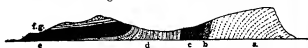
FIG. 1.—Section of the Isle of Wight—a Monoclinical Curve. a , Chalk; b , Woolwich and Reading beds; c , London clay; d , Bagshot series; e , Headon series; f, g , Osborne and Bembridge series.
