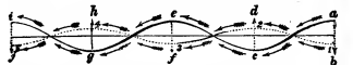
FIG. 29 shows how in progressive flight the wing and the body describe waved tracks —the crests of the waves made by the wing ( a, c, e, g, i ) being placed opposite the crests of the waves made by the body 1, 2, 3, 4, 5 .
