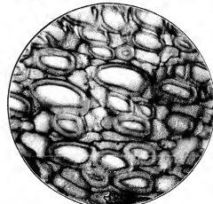
FIG. 6.—RAMIE. Section of bast region, \times 235 . Showing bast fibres bundles but only slightly occurring as individuals.
