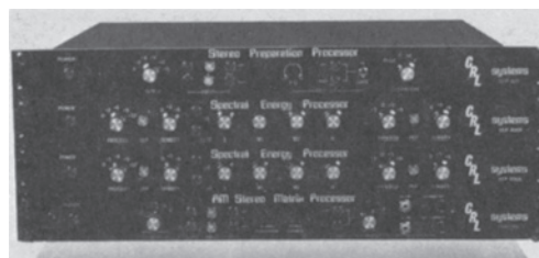
FIGURE 10.20 A station engineer must be knowledgeable about the sophisticated state-of-the-art audio processing equipment (such as the limiter and processor shown here) used by many stations, especially in metro markets where great sound gives a station an important competitive edge. Courtesy CRL Audio and Broadcast Electronics.
