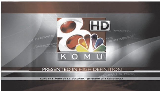
FIGURE 11.8 Essential graphics should stay within the middle of the television's scanning area. Note that this graphic can be used on 4:3 or 16:9 televisions. (Photo courtesy of KOMU-TV)
