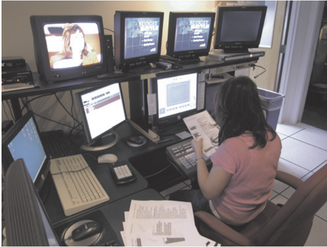
FIGURE 11.13 A standalone CG in use at a television station. (Photo by Jon Greenhoe)
