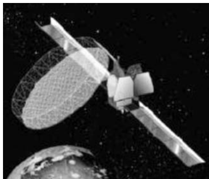
Figure 9.50 Artist's view of a geostationary satellite with a 12m unfurlable antenna. (Courtesy of Northrop Grumman.)
