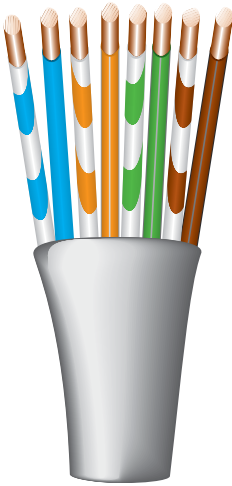
Figure 3-22 A Cat 5 UTP cable with pairs untwisted
