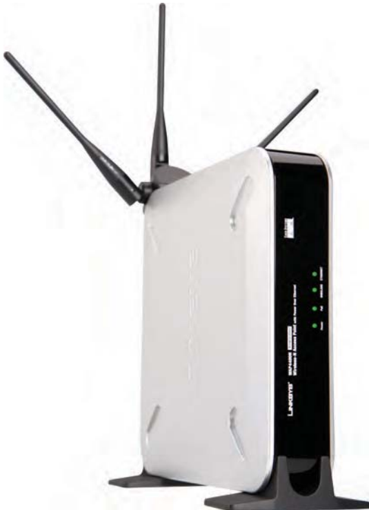
Figure 8-10 802.11n access point with three antennas
