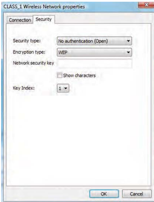
Figure 12-18 WEP selection in Windows Vista Wireless Network properties
