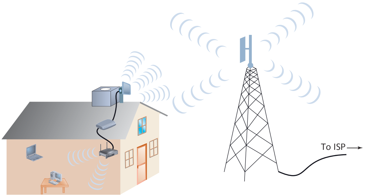
Figure 8-22 WiMAX residential service installation
