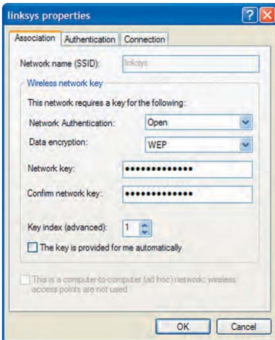
Figure 12-16 Entering a WEP key in the Windows XP wireless network properties dialog box
