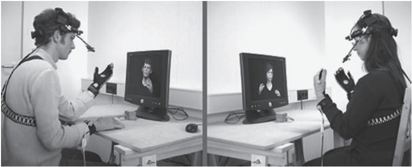
Figure 7.1 Base version of the avatar-based collaborative desktop environment (screen shot during calibration mirroring the interlocutor's own behavior).
