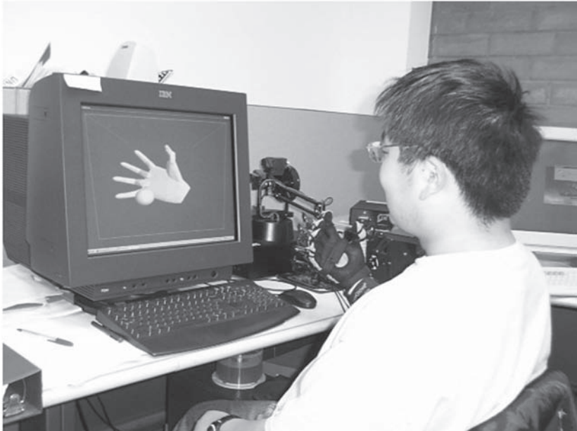
Figure 8.1 (a) User at location 1 uses a PHANTOM haptic stylus to touch the fingers of the user at (b) location 2, who is wearing a CyberGrasp haptic glove.
