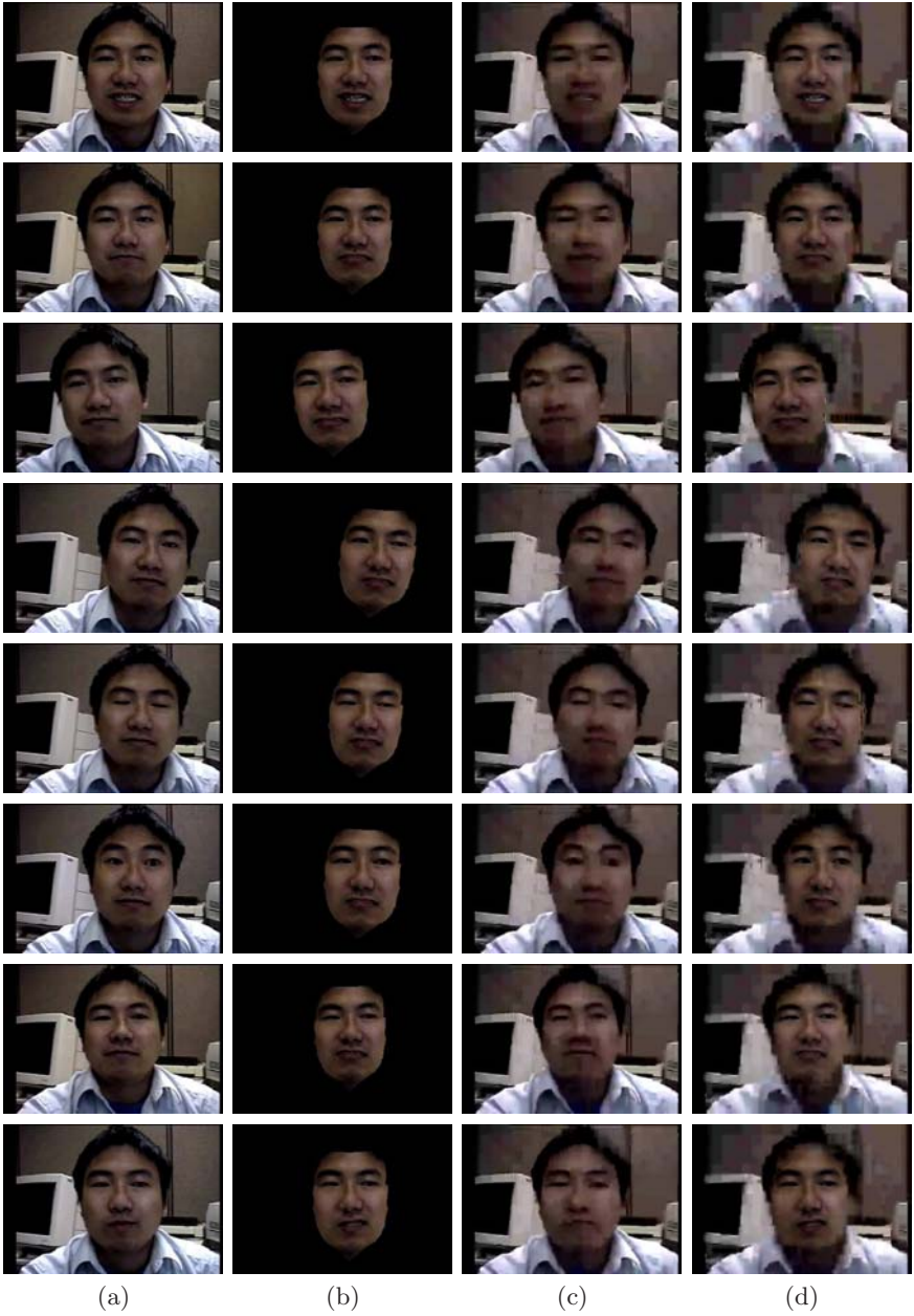
Fig. 21. Comparison of some video key frames. (a) The original frames; (b) The synthesized frames; (c) The H.26L decoded frames without face tracking; (d) The H.26L decoded frames with face tracking.
