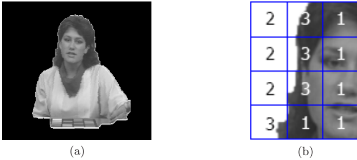
Fig. 3. Content-based coding scheme for arbitrary-shaped VO. (a) The binary alpha map. (b) The opaque, transparent, and boundary MBs
