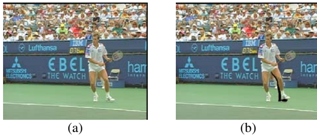
Fig. 23. Illustration of a typical scene concealment problem: (a) Original video scene; (b) Composition of two independently error concealed video objects (Soares and Pereira 2006c) (© 2006 IEEE).
