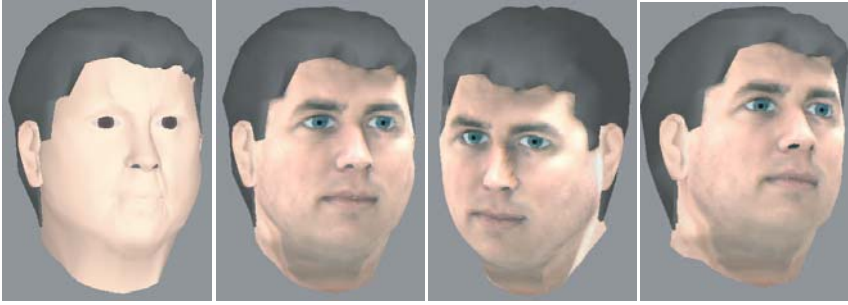
Fig. 10. Customized face model. (Left): Shape model. (Right): Texture is mapped onto the shape model which is rotated to several different poses. (Figure reproduced from [58] with permission.)
