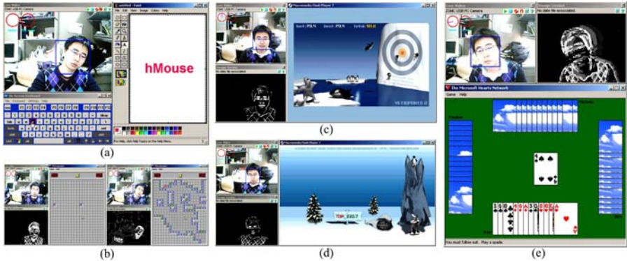
Fig. 3. On-screen typing and interactive games. (a) On-screen typing for Windows Paint text input. The text “hMouse” on the right Paint canvas is written by the hMouse typing on Windows on-screen keyboard shown in the lower-left part of the figure. (b) Playing Windows Minesweeper game with the hMouse. The left figure shows the cursor navigation while the right figure shows the left mouse button down and up click event. (c) Playing internet game, YetiSports 2 - Orca Slap [31], with the hMouse. (d) Playing internet game, YetiSports 1 - Pingu Throw [30], with the hMouse. (e) Playing Windows Hearts game with the hMouse.
