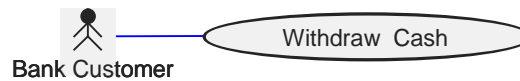
Figure 13. UML only explicitly addresses stakeholders inside our system with its use case actors
