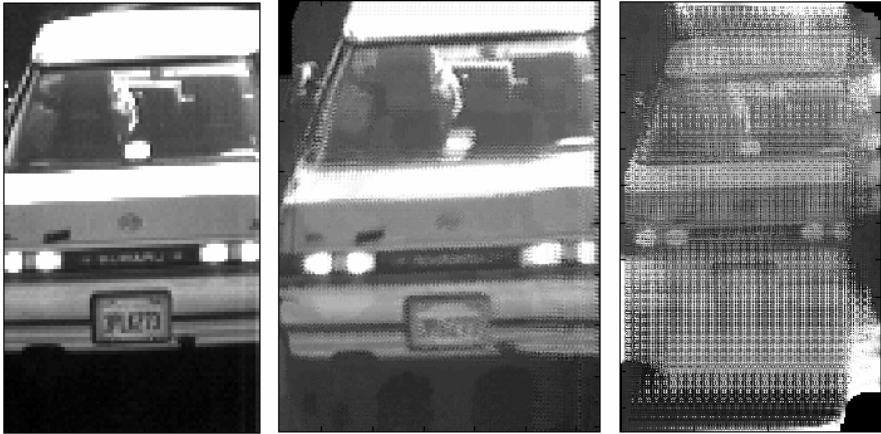
Fig. 10.1 (a) LR source image, (b) SR image, (c) SR image with motion estimation errors
