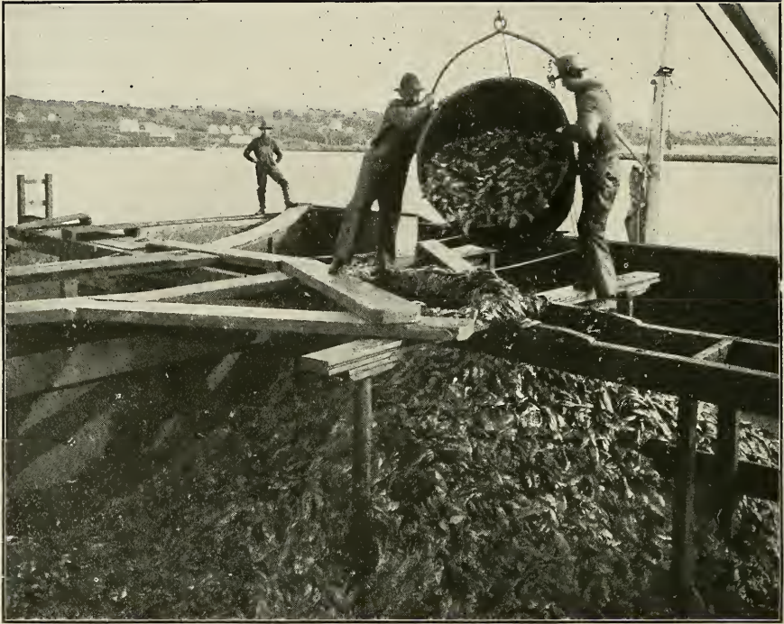
Discharging Menhaden from Vessel by Means of Tubs
