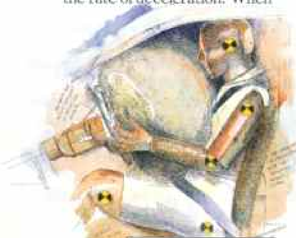
Driver-side air bag. Inflates in 50 milliseconds.
