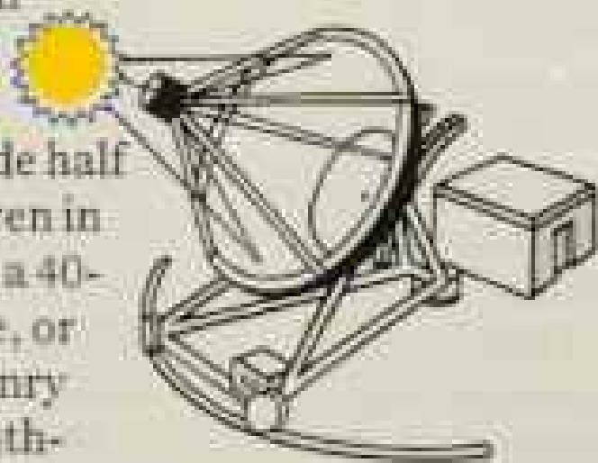
1 Tracking concentrators follow the sun on its course. The reflective dish concentrates solar radiation to produce electricity directly through photovoltaic
