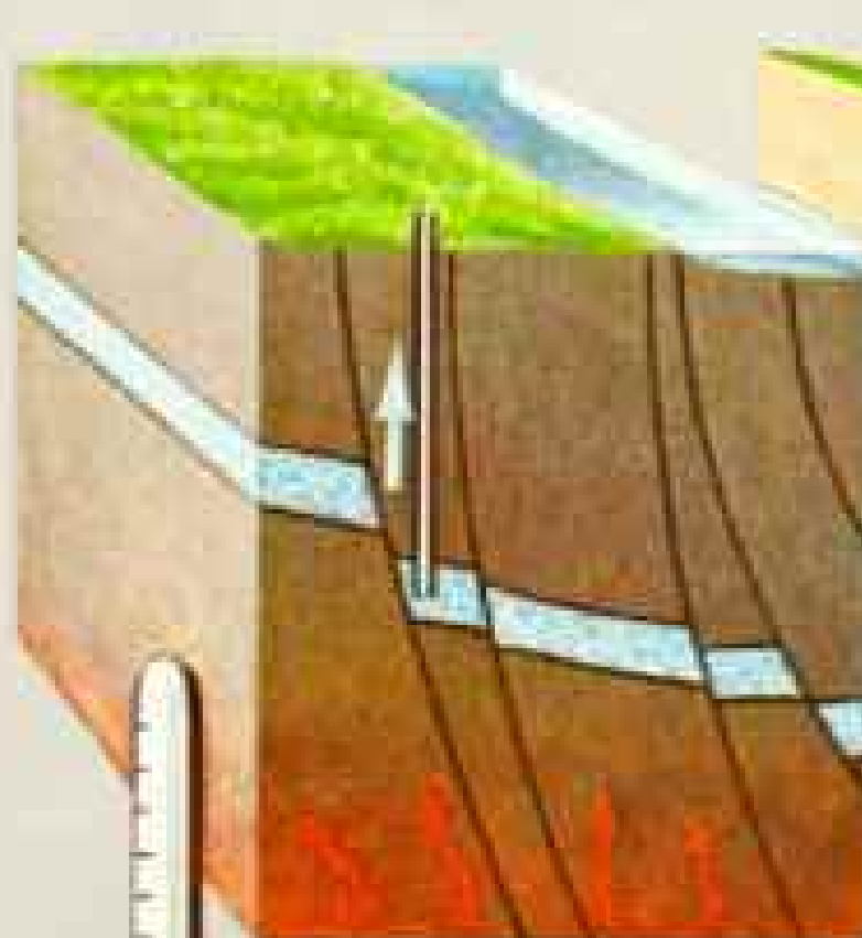
Water and methane are trapped in porous rock layers which are sandwiched between shale in geopressured zones. Gas is the main prize, hot water the second.
