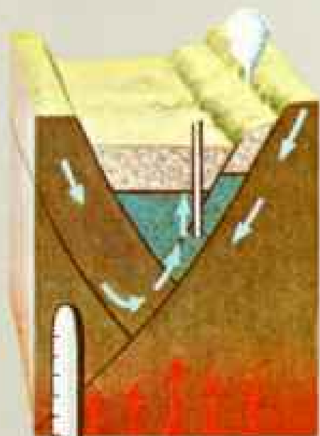
Cool water seeps toward the earth's warm interior. Heated, it returns along fractures to vent or become trapped under impermeable layers where wells can recover it.
