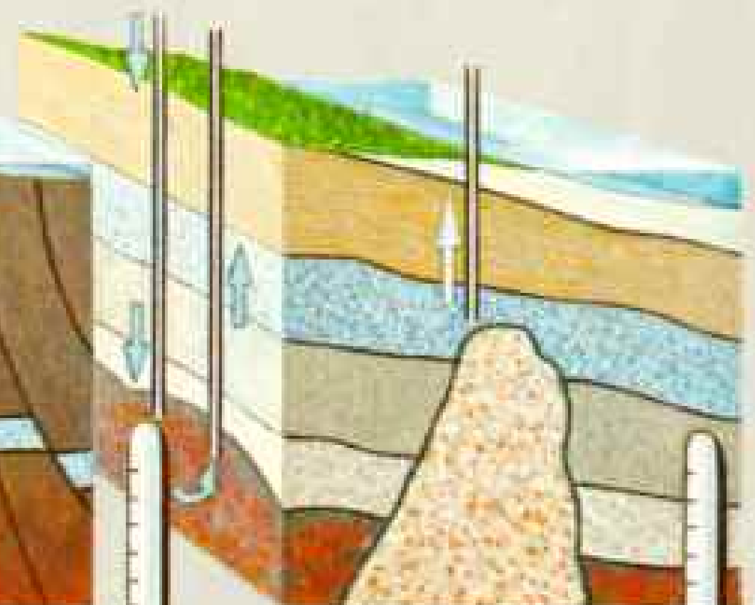
Water pumped down into hot dry rock (left) circulates through fractures, picking up heat for recovery at the surface. Radioactive granite intrusions (right) offer favorable geothermal sources.
