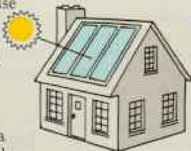
2 Flat-plate thermal collectors carry tubes filled with air, water, or other fluids. In the Northern Hemisphere, collectors are most effective on roofs and when facing
