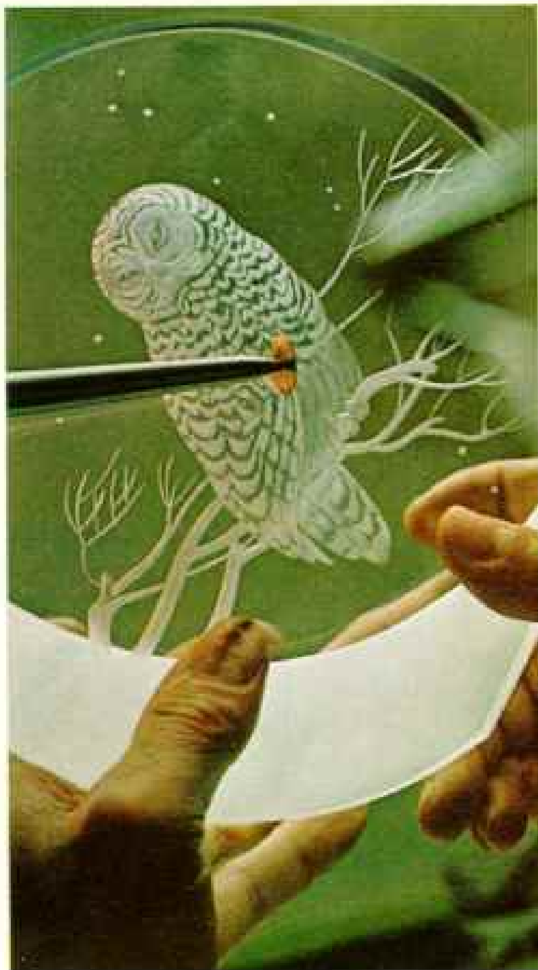
Delicate strokes from a copper engraving wheel complete a crystal disk at the Steuben Glass factory in Corning. The barred owl, in an edition of only 30, costs $6,100. Each may take 200 working hours.
