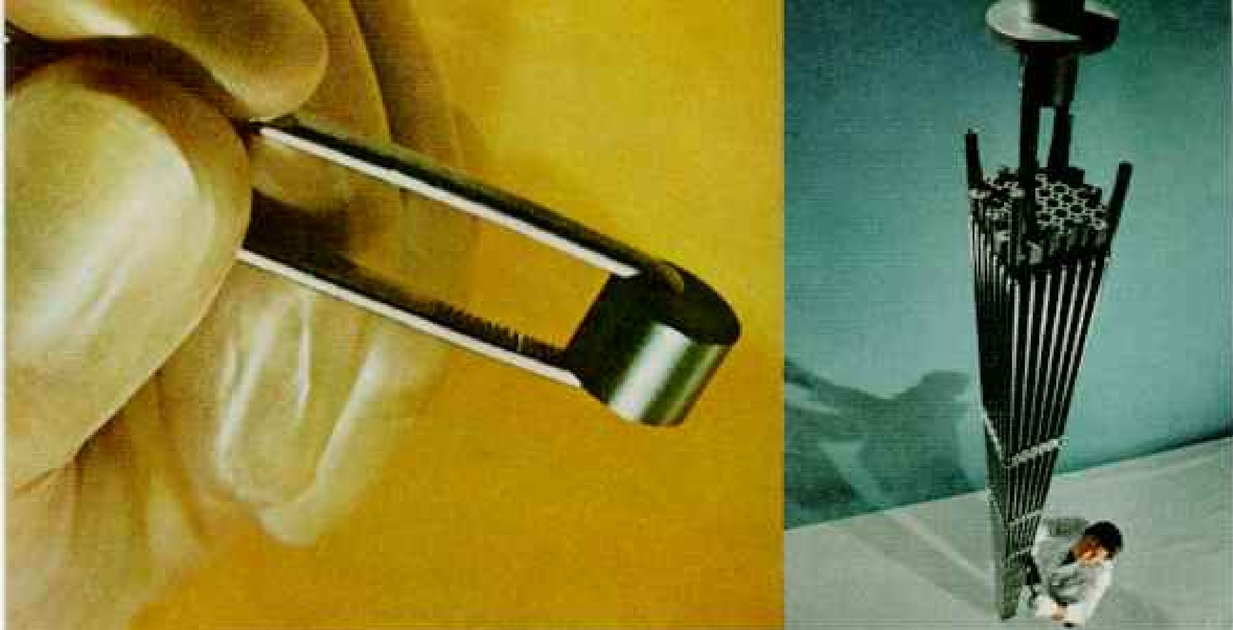
Pellets of enriched uranium (left) and fuel assemblies (right) are made by Exxon Nuclear Company. The pellets are inserted into rods, and the rods are grouped to form assemblies which make up the core or "furnace" of a nuclear reactor. An assembly, like the one shown, can generate enough electricity to run 16,000 average homes for a year.
