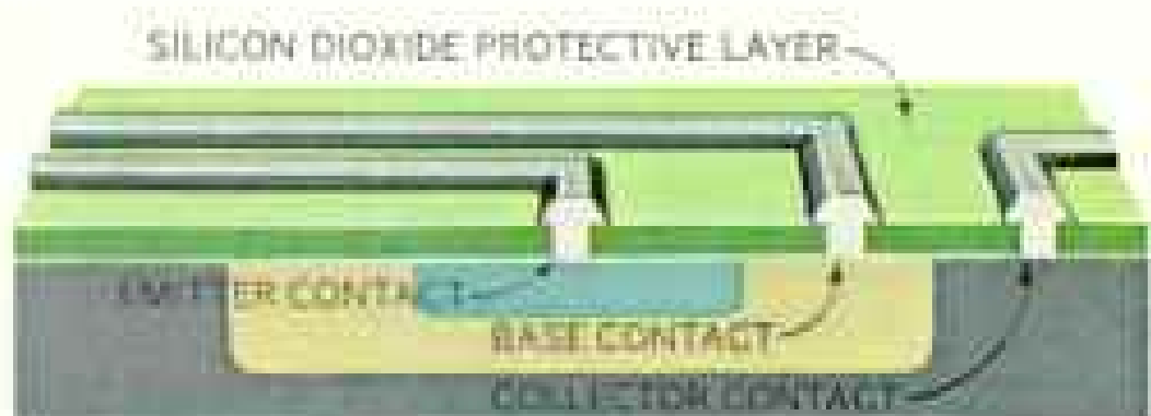
Simplified diagram shows a transistor in cross-section
