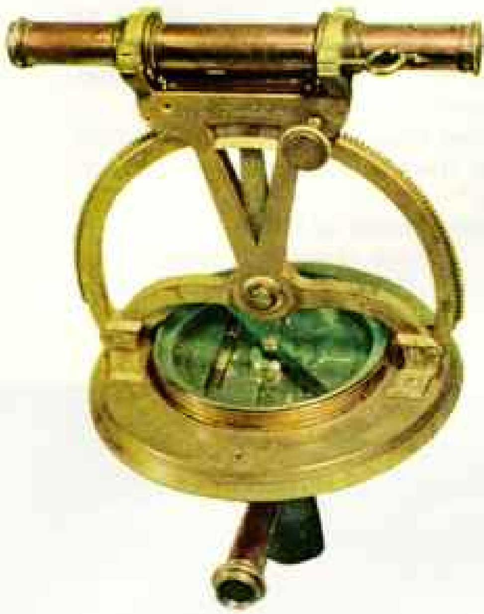
Measuring the countryside around his estate, Jefferson used this theodolite to sight on nearby peaks.
