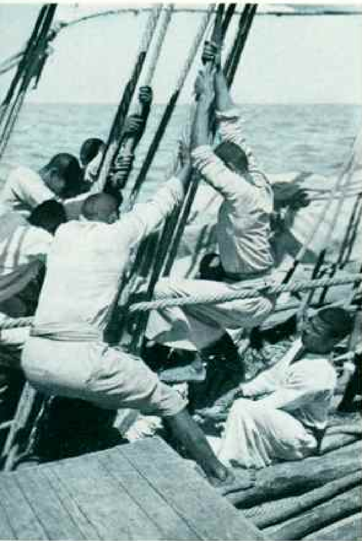
Barefoot Sindhads haul on halyards after sheeting home a lateen sail aboard a Kuwaiti boom. They hoist the sail and swing the yard by hand.
