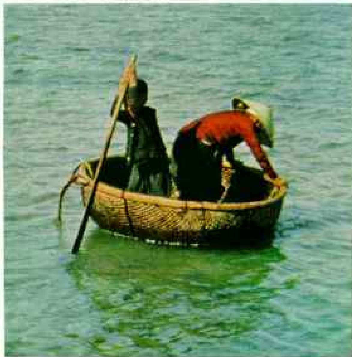
Bamboo basket boat in South Viet Nam lacks bow or stern but makes headway. Calking with cow dung and coconut oil waterproofs the craft.
